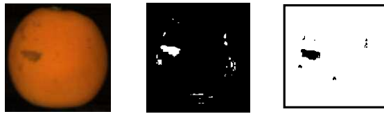
Fig. 76. Blemish identification testing for blemished ripe orange.
