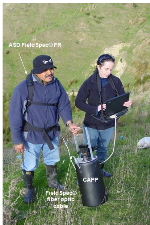
Figure 4.1. Collection of canopy pasture spectral data using the CAPP attached to an ASD FieldSpec ® Pro FR.
