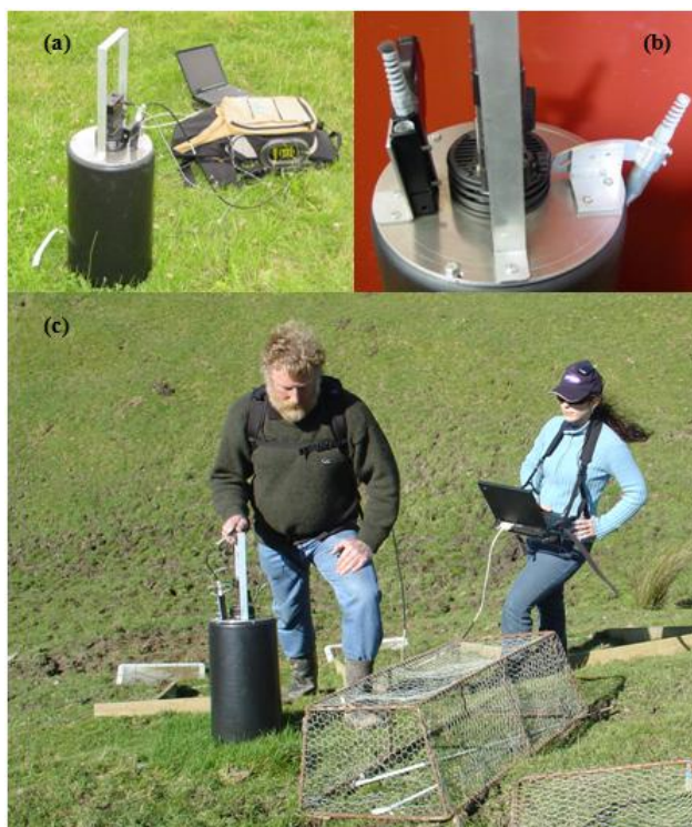
Figure 2.1. (a) CAPP with the spectroradiometer ASD FieldSpec® Pro FR; (b) ASD light source mounted on the top and fibre optic cable grips on the top and side of the CAPP; (c) acquiring reflectance spectra from sheep-grazed pasture.
