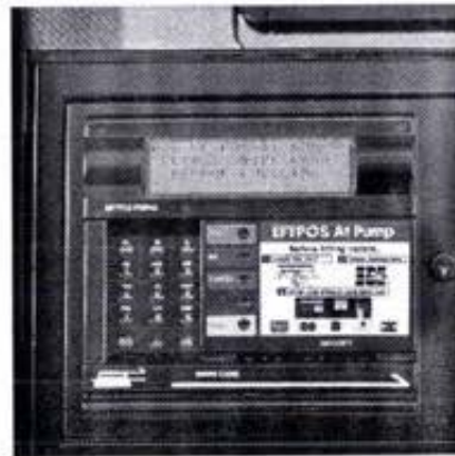
Figure 2.1: Current Forecourt Service Terminal (FST)
