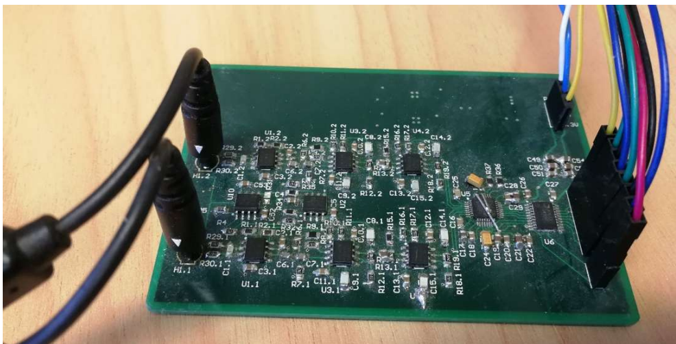
Figure 3-36. The fabricated EMG signal acquisition circuit PCB.
