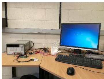
Figure 6-13. The pattern recognition-based real-time EMG-driven five-fingered robotic hand system.
