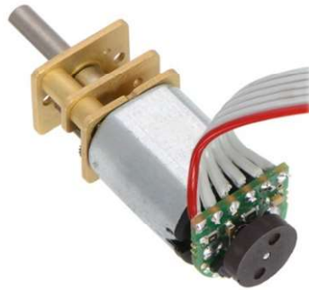
Figure 5-17. The magnetic encoder from Pololu attached to a Pololu brushed DC motor.
