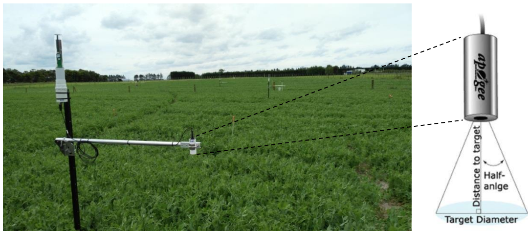
Figure 3.2: Typical infrared thermometers sensor arrangement in peas crop (site A) for measuring the crop stress. The infrared thermometers mounted at 0 degrees below horizontal which give a visible area of 1.2 \text{m}^2 .
