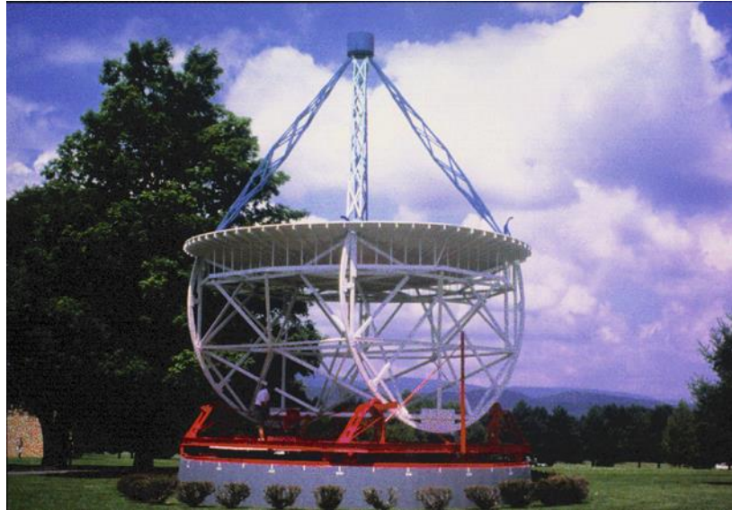
Figure 2-1: Grote Reber's 9m diameter Parabolic antenna remains in National Radio Astronomy Observatory (NRAO) as a historical monument [9]. First Radio telescope used for astronomical research.
