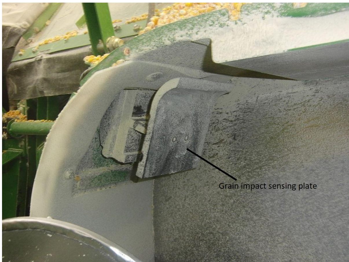
Figure 3-2 Yield monitor based on the measurement of mass grain flow (the sensing plate converts the impact of the incoming grain into electric signals)
