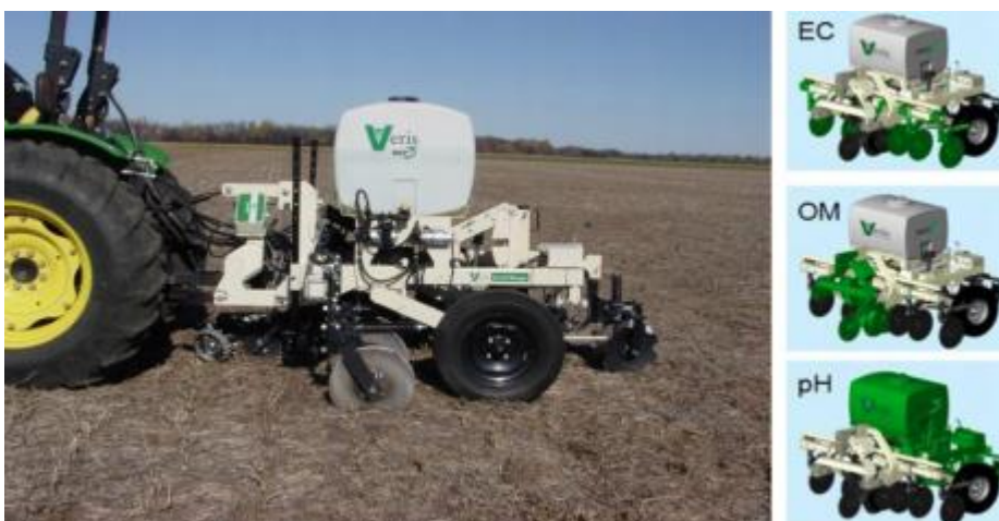
Figure 3-3 Veris Mobile Sensor Platform (MSP-3) (Source: Hurst et al., 2015)
