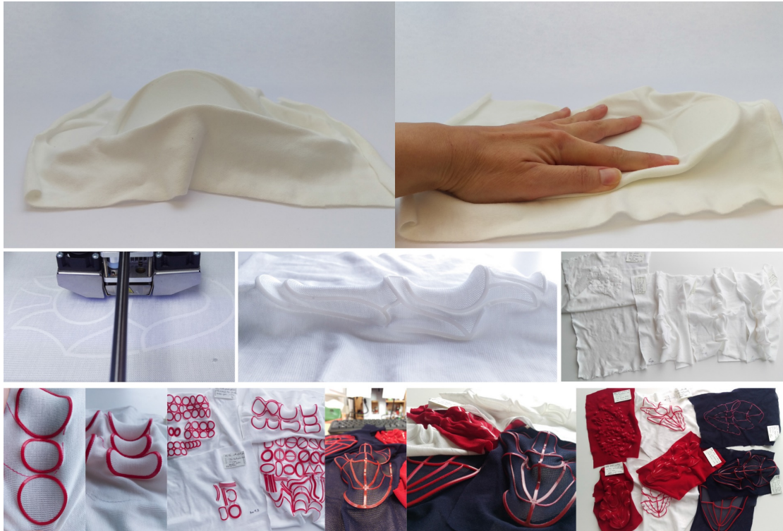
Fig. 4. 6. Stress exploration as one of promising collapsibility principles. 3D prints with TPU on stretched fabric.
