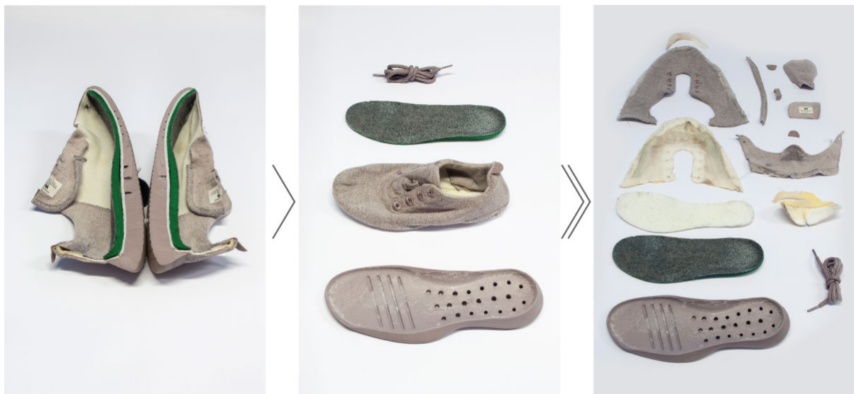
Fig. 3. 14. Images showing the components and reverse assembling steps.
