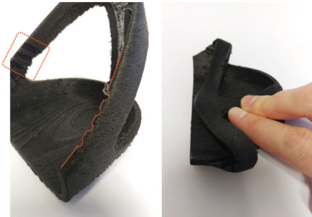
Fig. 4. 22. Testing heel “smooshes” performance.
