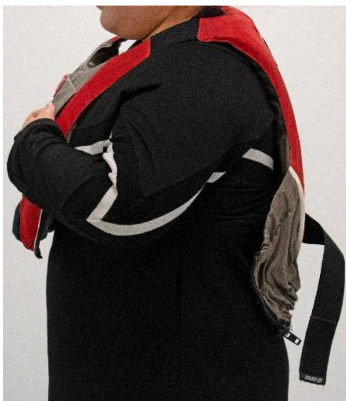
Figure 6.17: E3 (aquatic sports) life jacket is too small for participant 3 to properly donn
