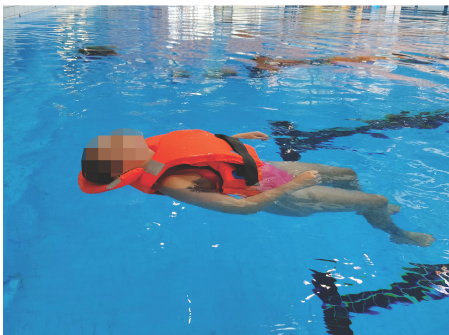
Figure 38: Aquatic trials conducted with the R6 life jacket prototype with minor modifications
