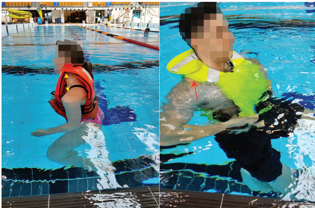
Figure 7.7: Comparison of shoulder rise between Existing life jacket and Slot n' Slide panel life jacket
