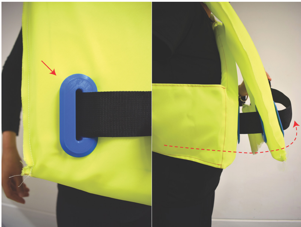
Figure 6.27: 3D printed guides inserted into the crossover front panels; Webbing strap is passed through the guides in the under and upper crossover panels
