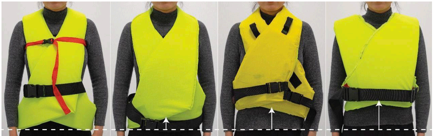
Figure 6.10: Reduction of life jacket height in subsequent iterations.
