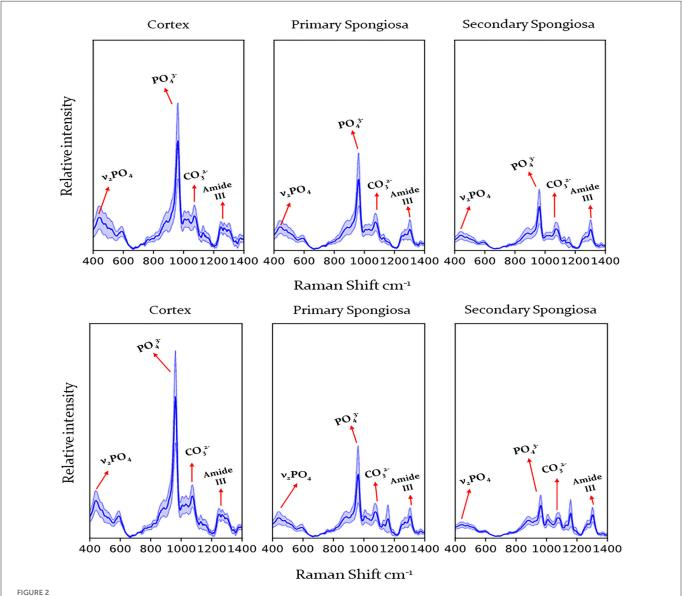
Raman spectra obtained from the humerus from cows with humeral fracture (**upper graph**) and control cows (no fractures) (**lower graph**) by location (cortex, primary, and secondary spongiosa). Labels indicate peaks used for calculation of mineral/matrix ratio, carbonate/phosphate ratio and crystallinity. Dark line indicates mean, pale blue line 95% confidence interval.  $PO_4^{3-}$ , phosphate;  $CO_3^{2}$ , carbonate.
