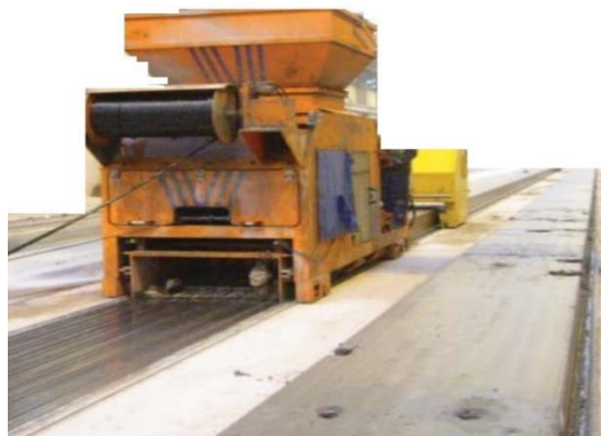
Figure2. 16: Oval voids hollow core machine with slip-forming technique
