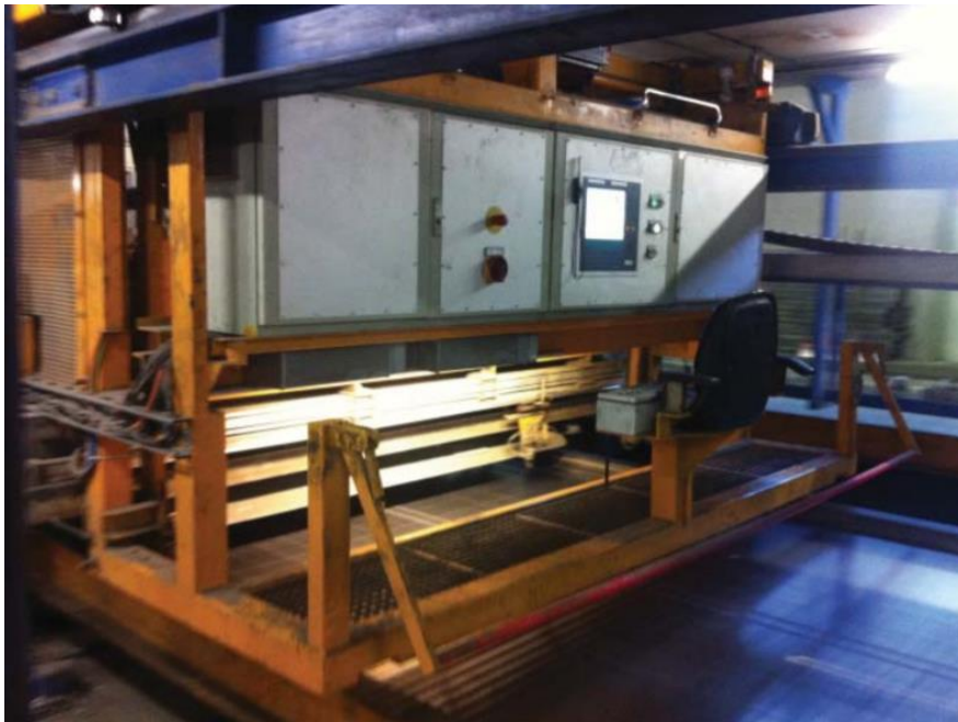
Figure2. 10: First shuttering machine within a pallet-rotation plant.
