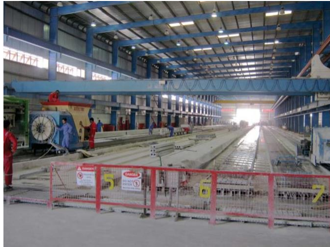
Figure2. 15: Hollow core slab production (using extrusion method)
