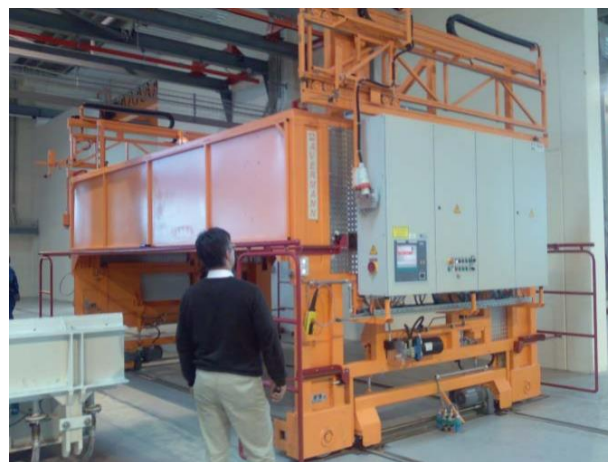
Figure2. 14: pre-stressed floor production on the long bed with plotting device
