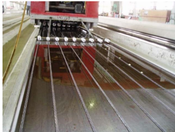
Figure2. 17: Circular voids hollow core machine with extrusion technique
