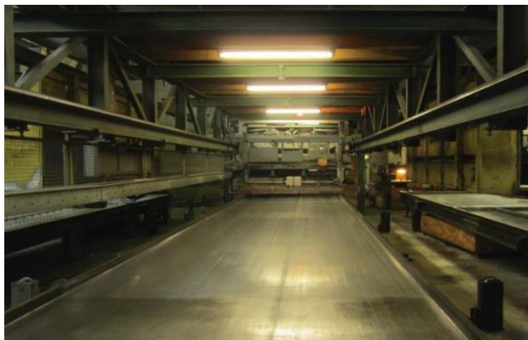
Figure2. 9: An early pallet circulation system for precast concrete wall panels
