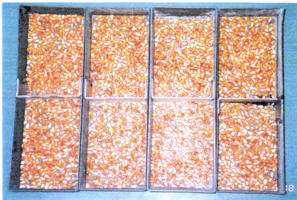
Plate 3-3. Arrangement of maize grains in a single layer in the drying trays before drying.
