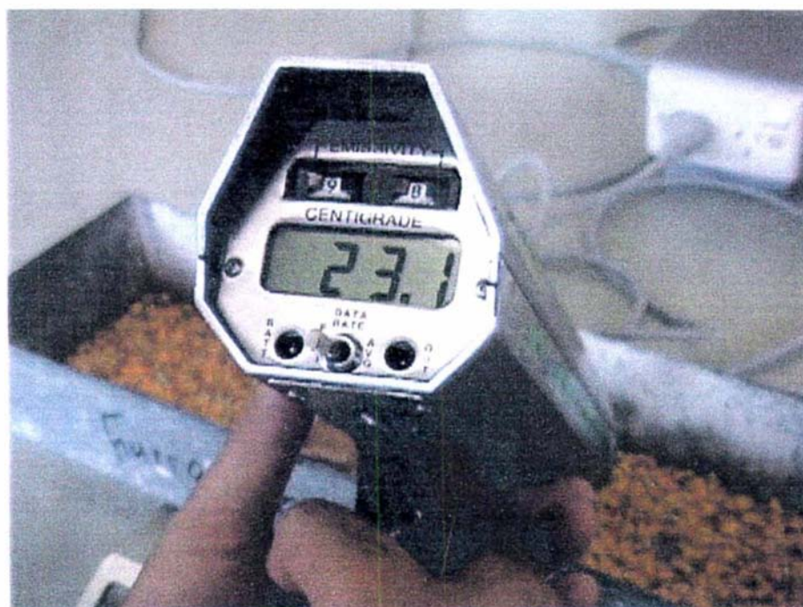
Plate 3-4. An example of measuring an instant grain surface temperature by using an infrared thermometer (The infrared thermometer in this photo indicates a surface grain temperature of 23.1°C, the air temperature was 25°C).
