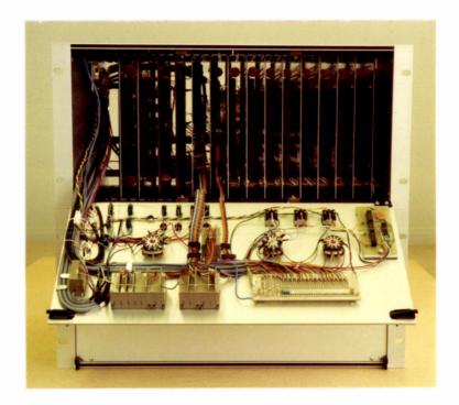
Figure 3.2 Front view of correlator with control panel open.
