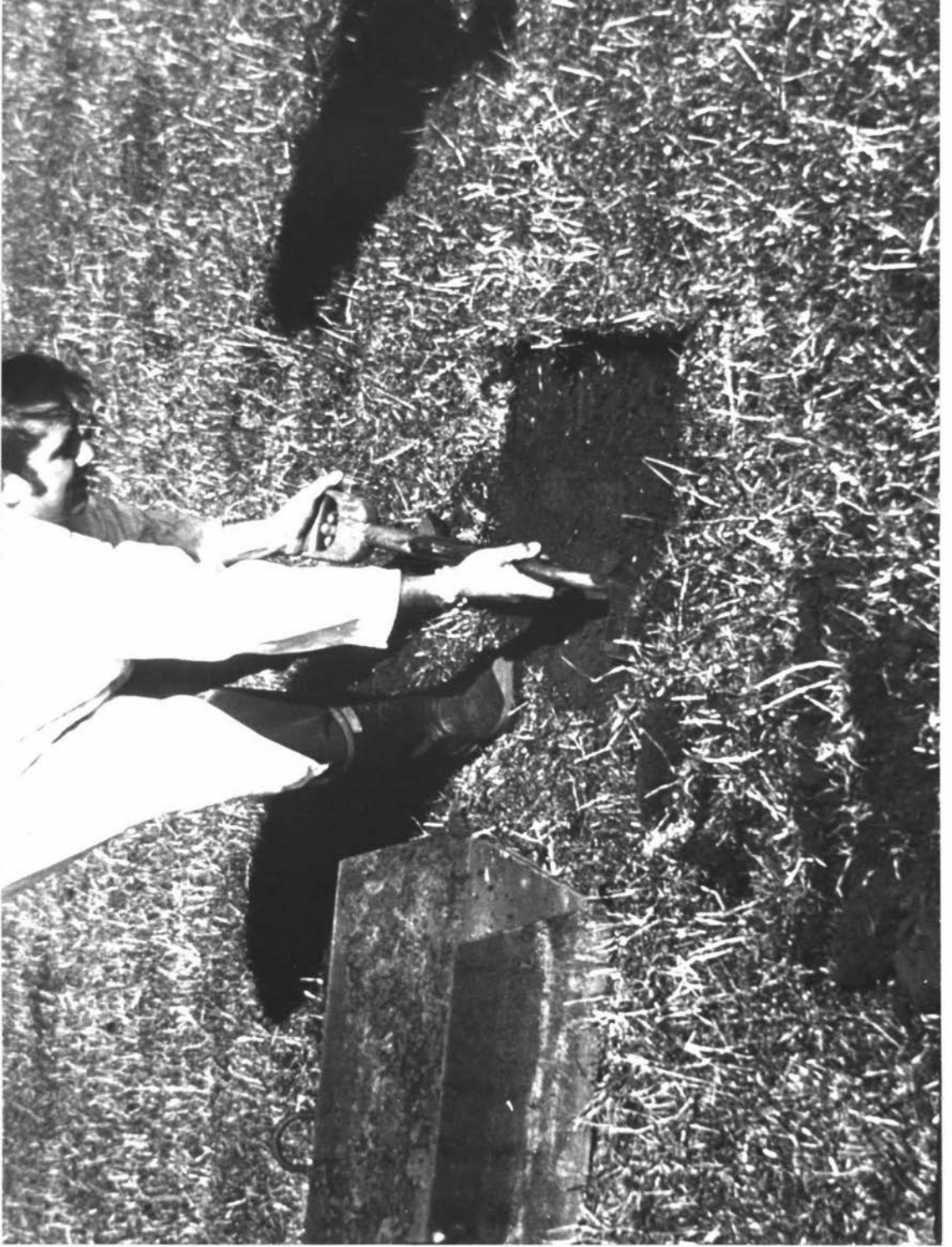
Plate 6: Turf block extraction procedure; (1) cutting lead-in channel
