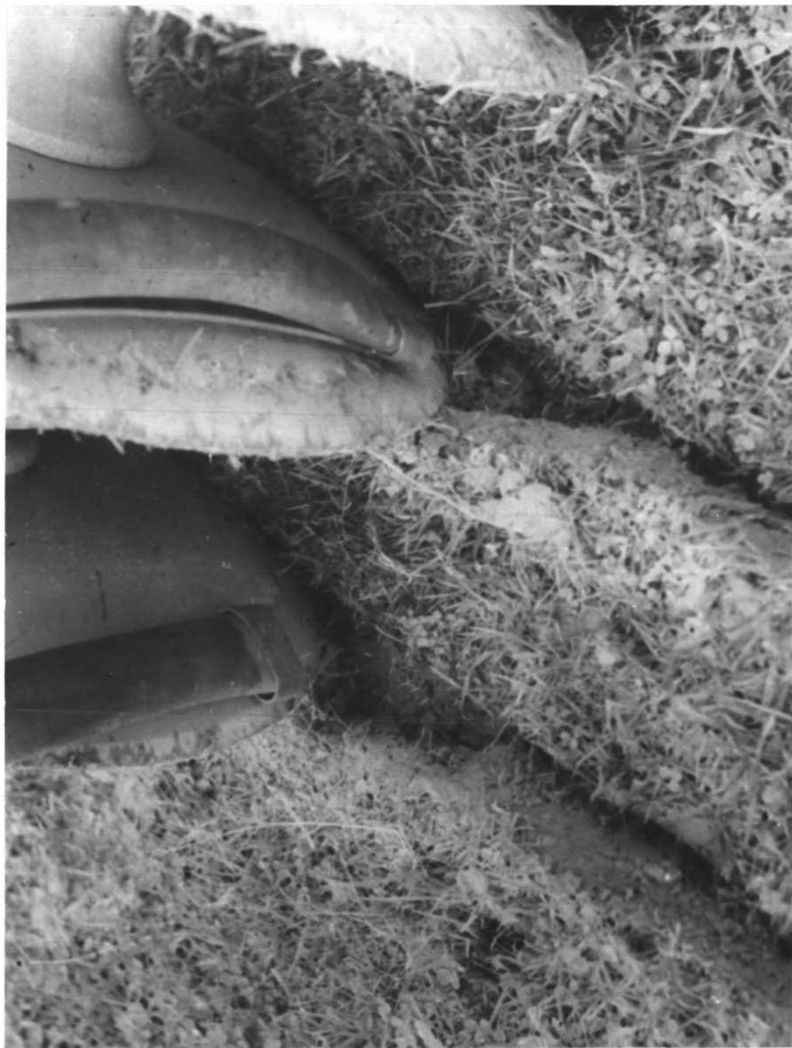
Plate 2: Dished disc coulters creating soil flaps in moist soil
