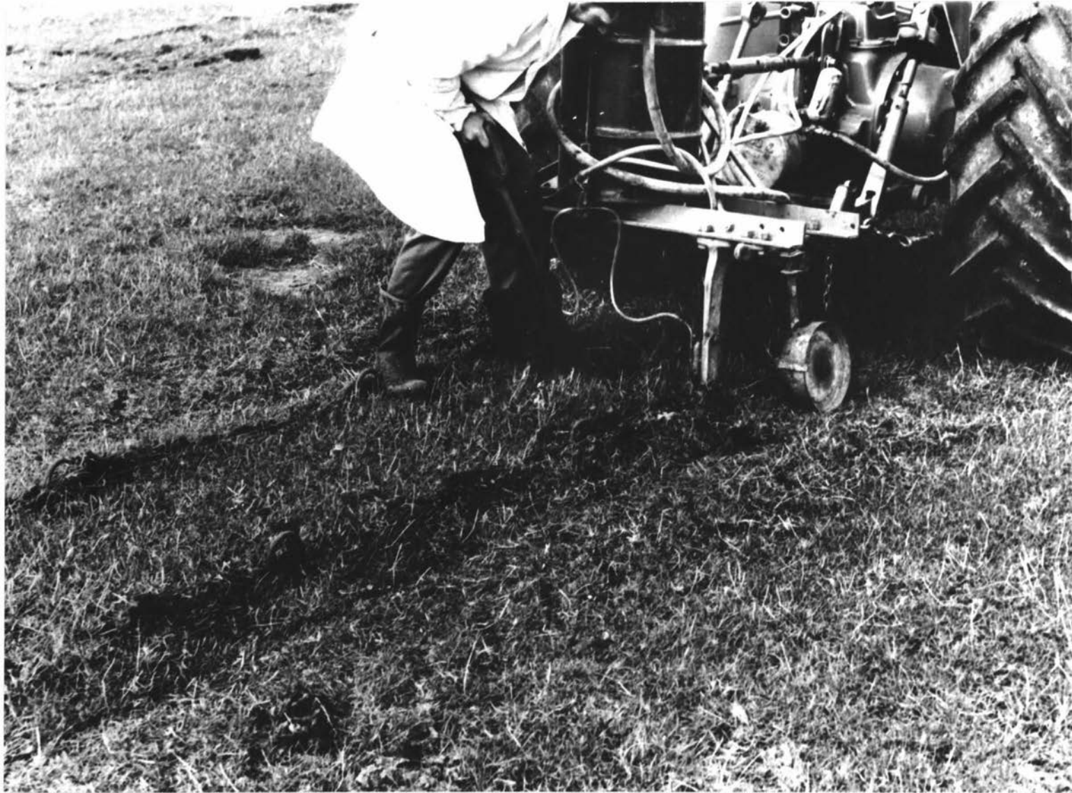
Plate 11: Turf block extraction procedure; (6) severing the turf block ends
