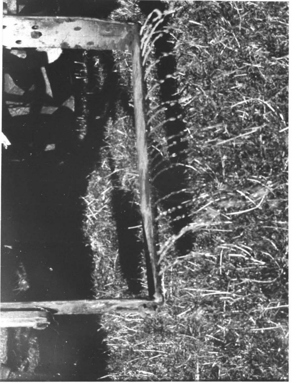
Plate 5: Water discharge from the hollow turf cutter blade
