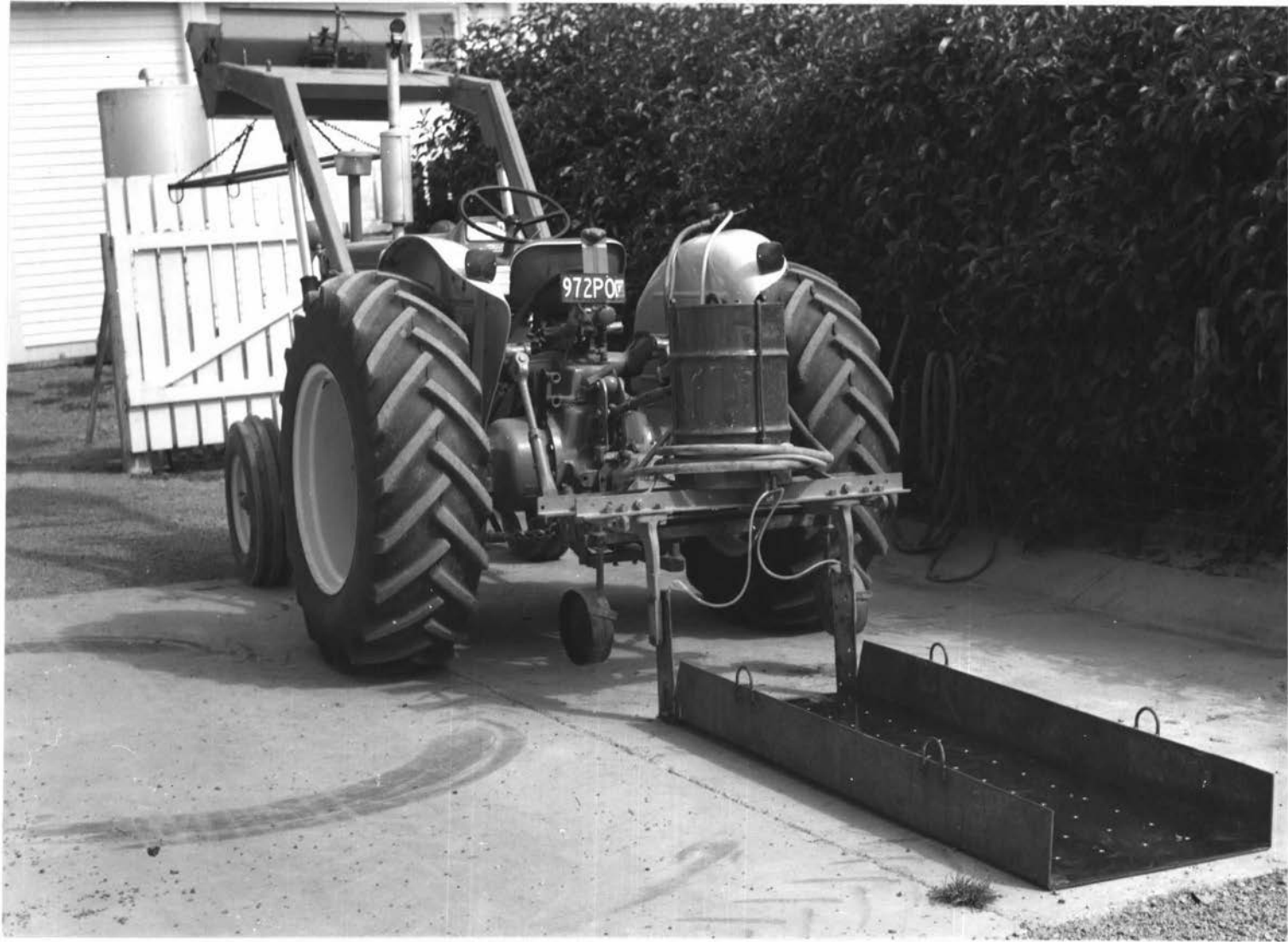
Plate 4: The turf cutter with a tillage bin attached
