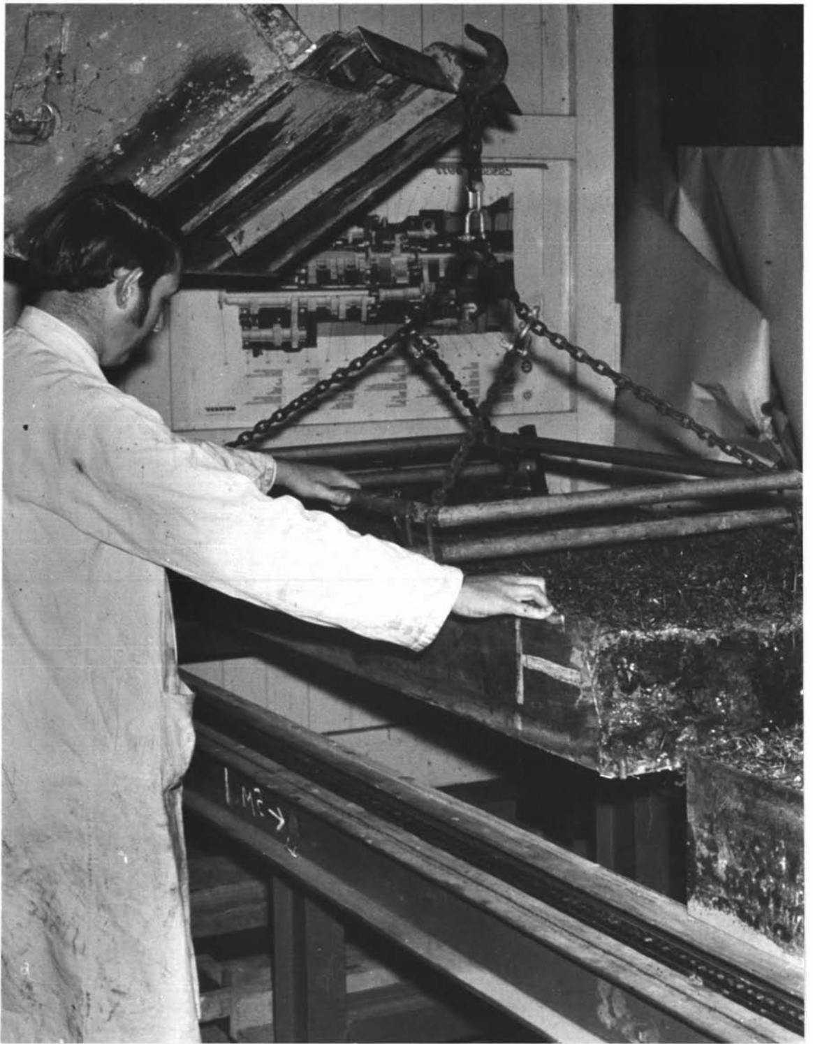
Plate 17: Placement of a tillage bin on the support bed
