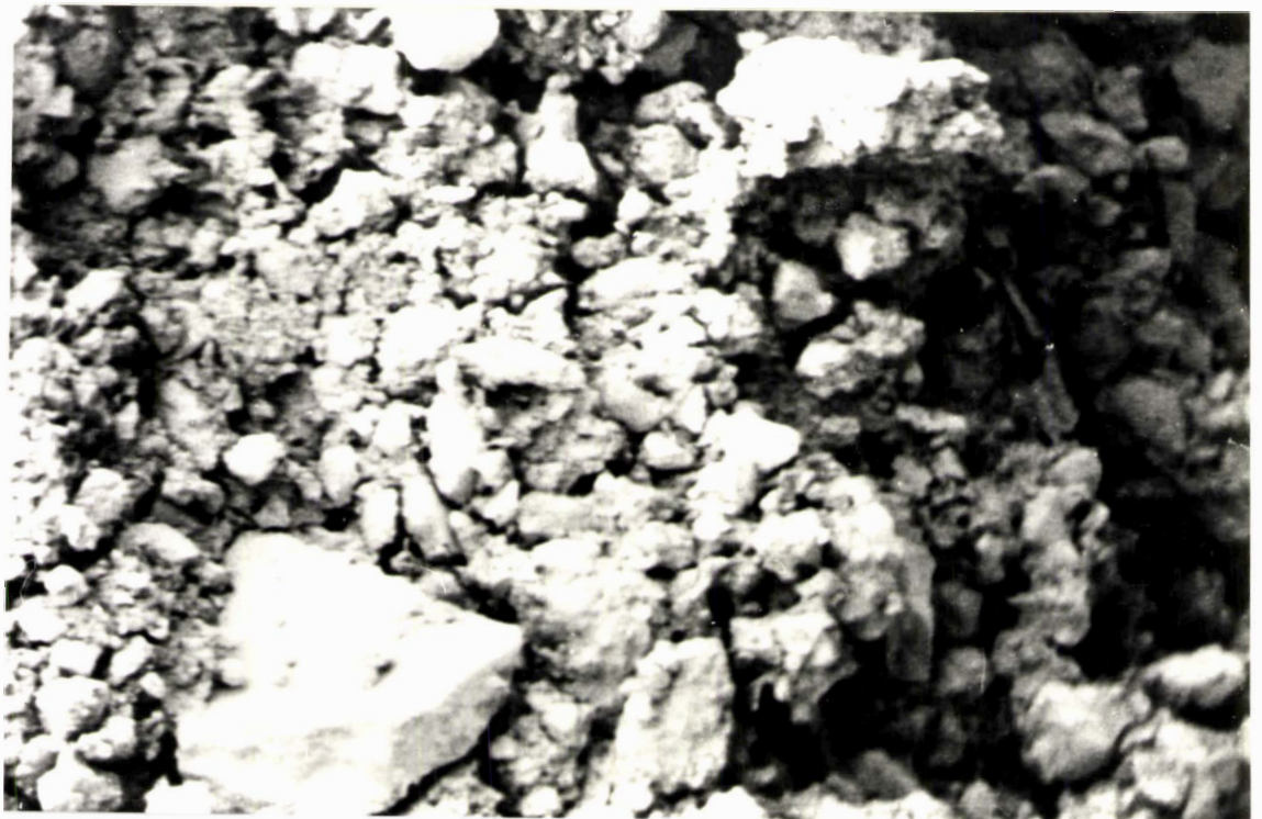
Fig.46. Micrograph(x170) taken 20-30mm from the soil/chisel coultter interface.
