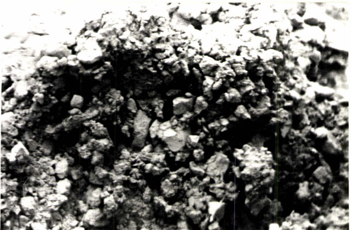
Fig.44. Micrograph(x170) taken 10-20mm from the soil/chisel coultter interface.
