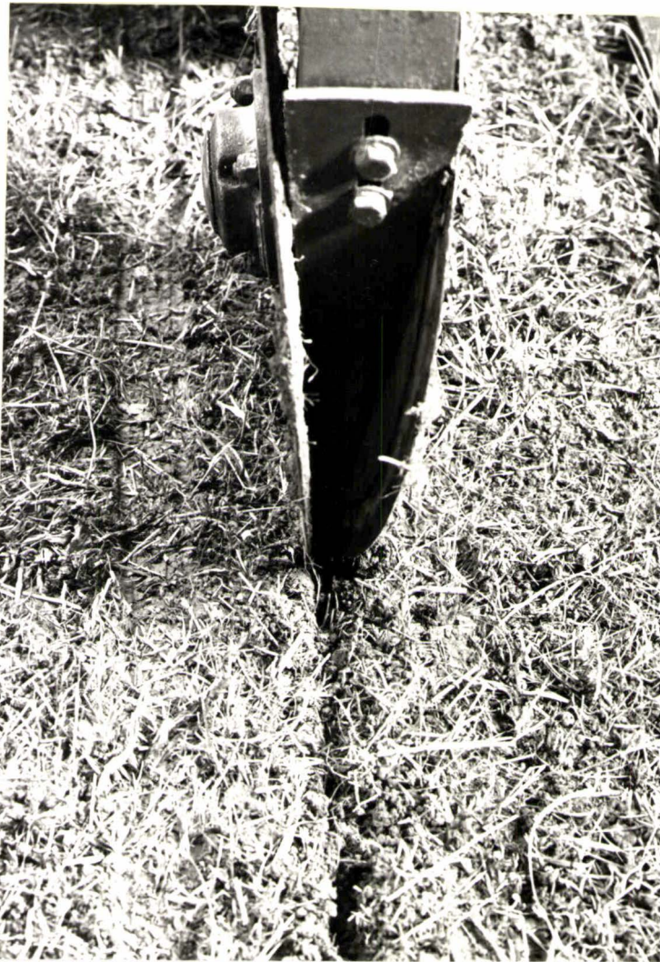
Fig.61. The characteristic shaped groove of the Triple disc coultter.
