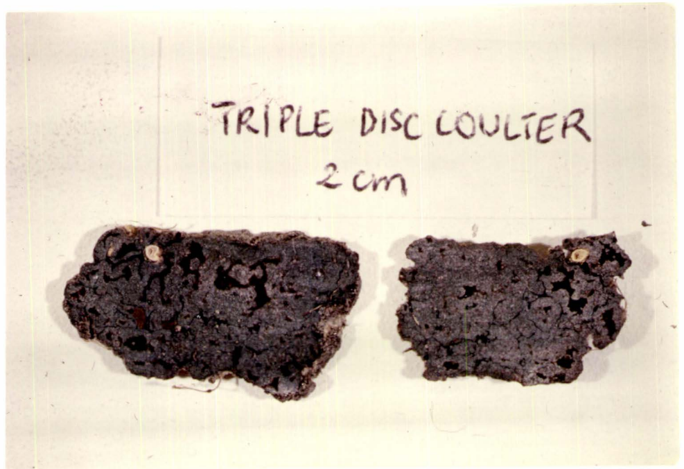
Fig.35. Soil sections taken at 20mm from the soil/triple disc coulter interface.
