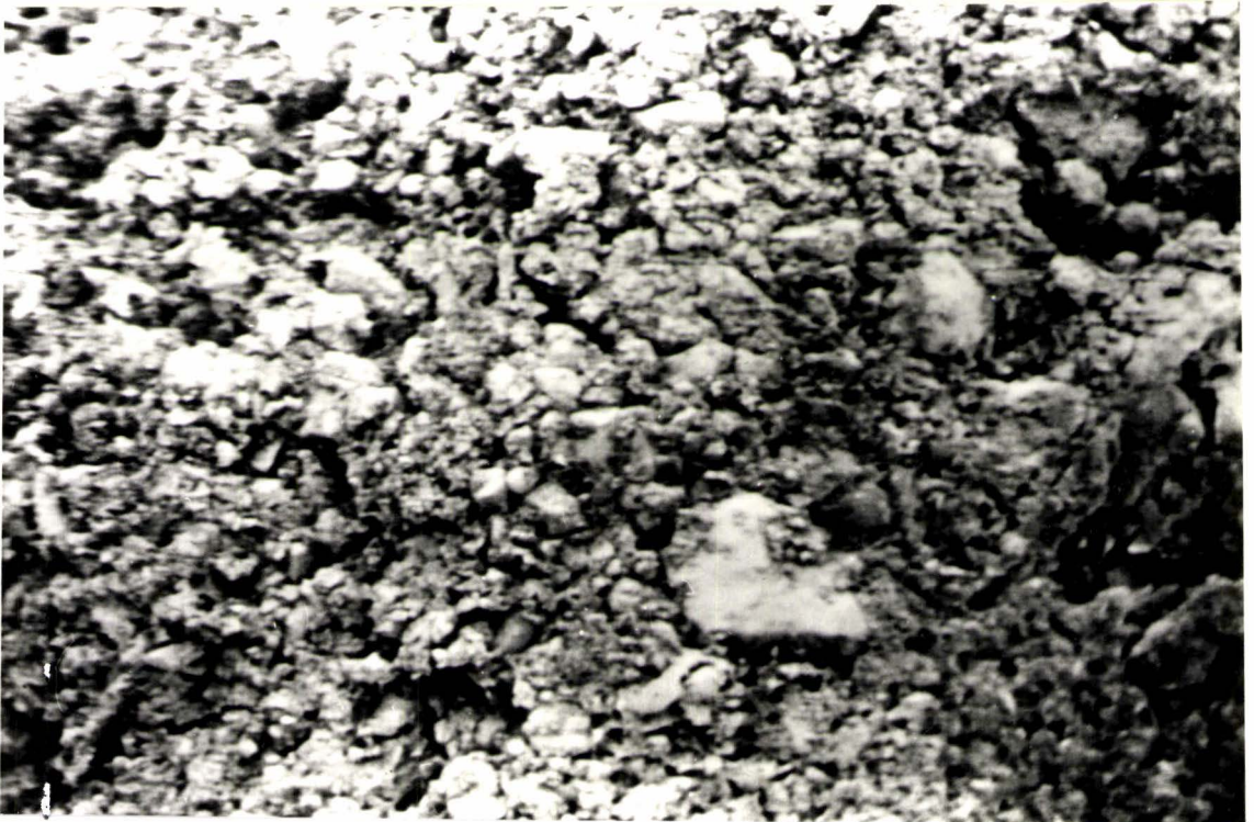
Fig.43. Micrograph(x170) taken 10-20mm from the soil/triple disc coultter interface.
