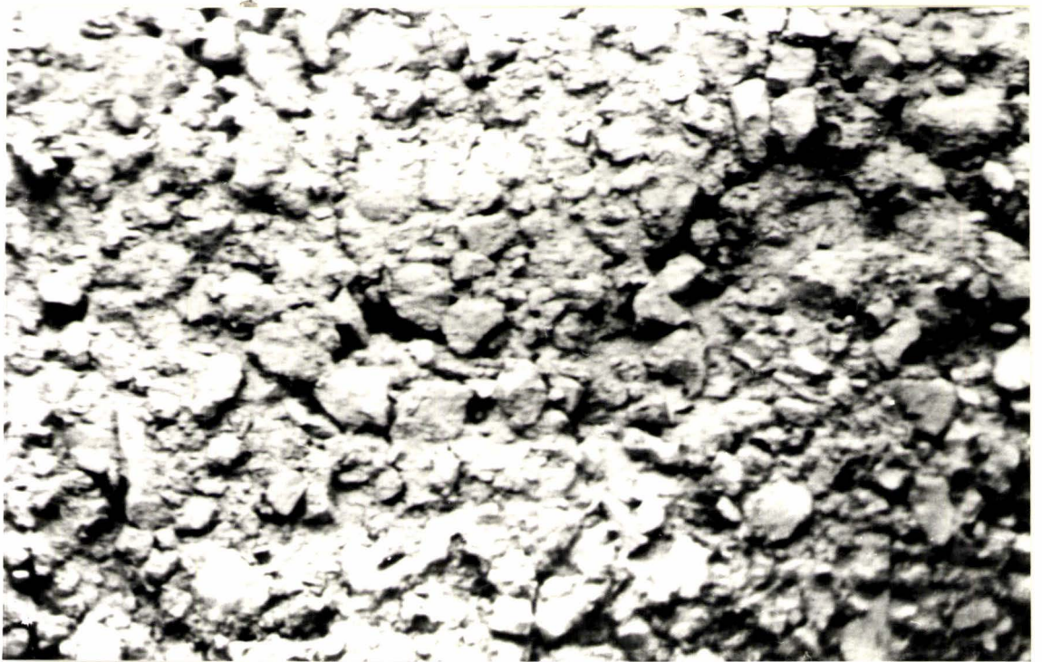
Fig.47.Micrograph(x170)of a soil at the base of the triple disc coultter created groove.
