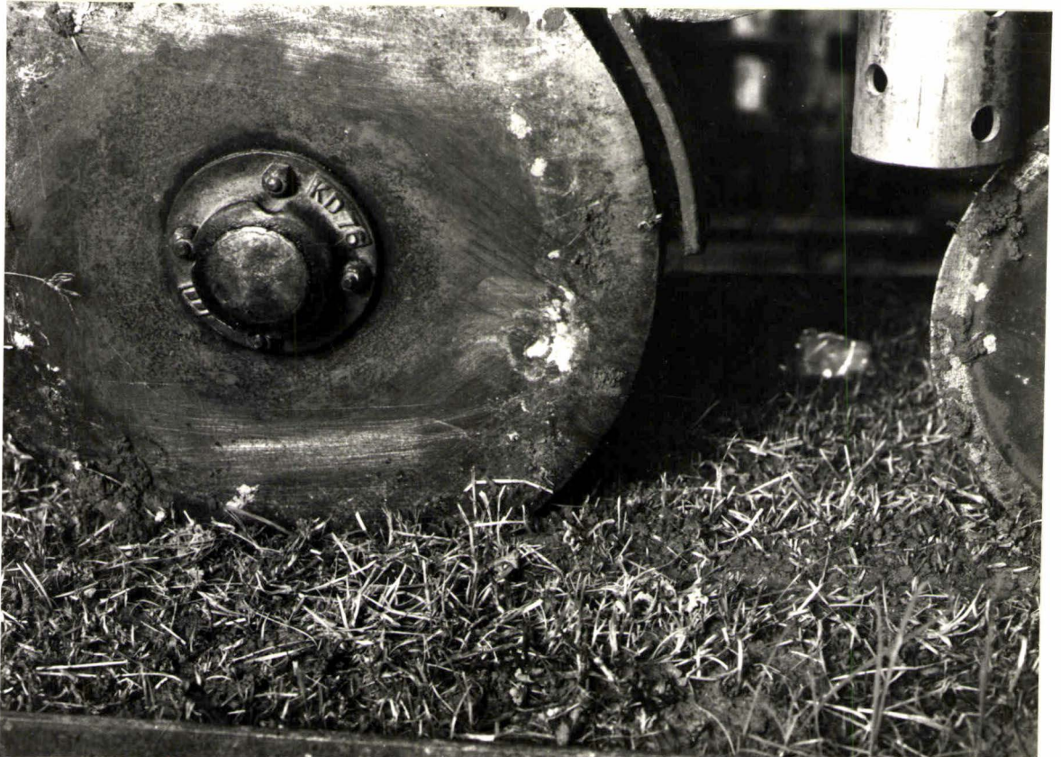
Fig.53.The triple disc coulters has a greater longitudinal soil/coulters contact.
