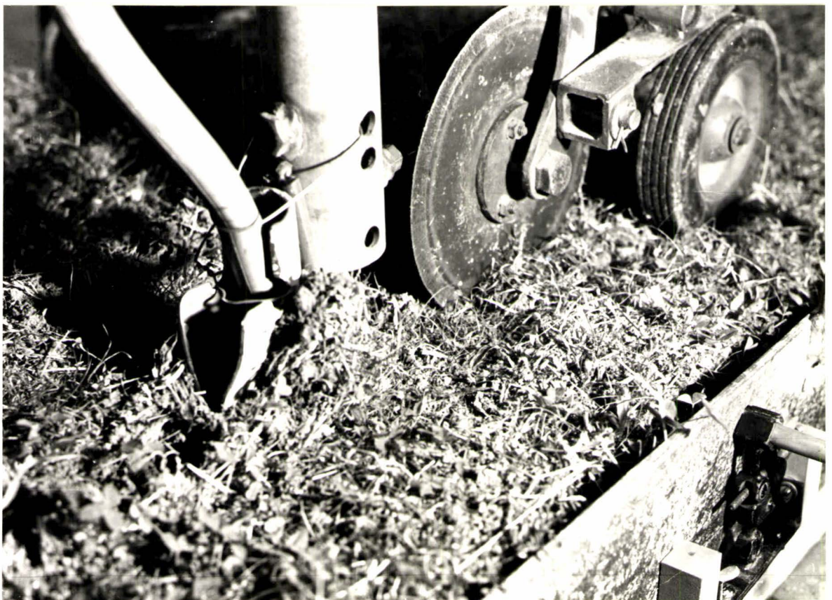
Fig.54.The chisel coulters shatters soil abruptly on both sides of the coulters.
