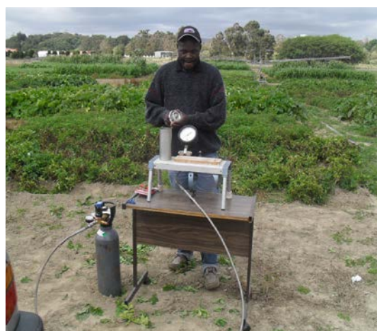
(b) Leaf water potential measurements by Pressure chamber
