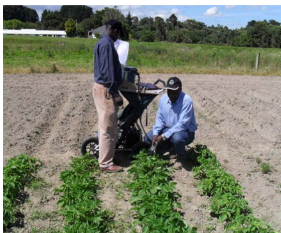
(a) Gaseous exchange measurements by CIRAS - 2
