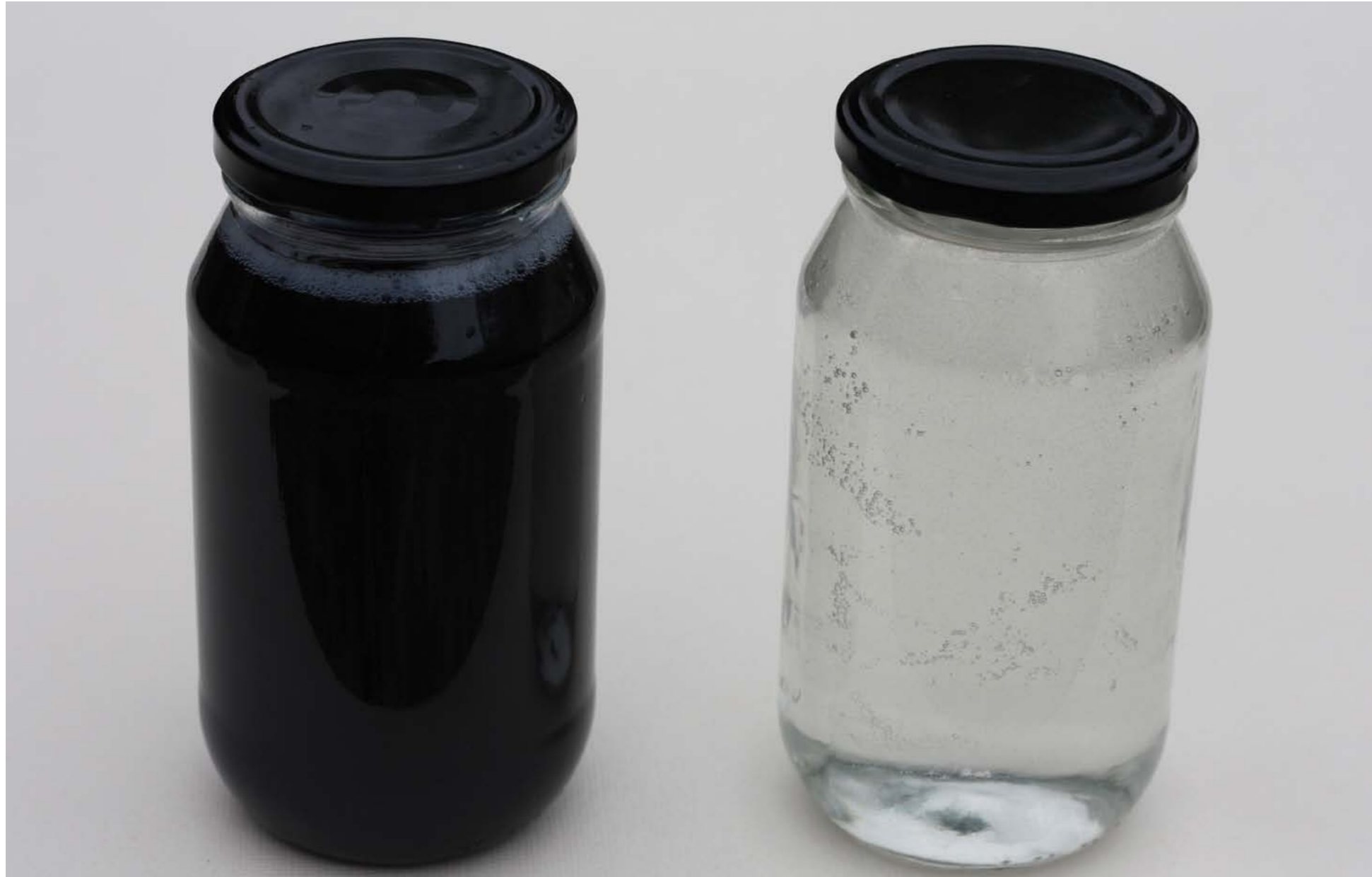
Figure 19: Left jar contains Navy dye powder that did not exhaust properly in the dye bath, right jar contains the same Navy dye powder properly exhausted at the end of the dye bath.
