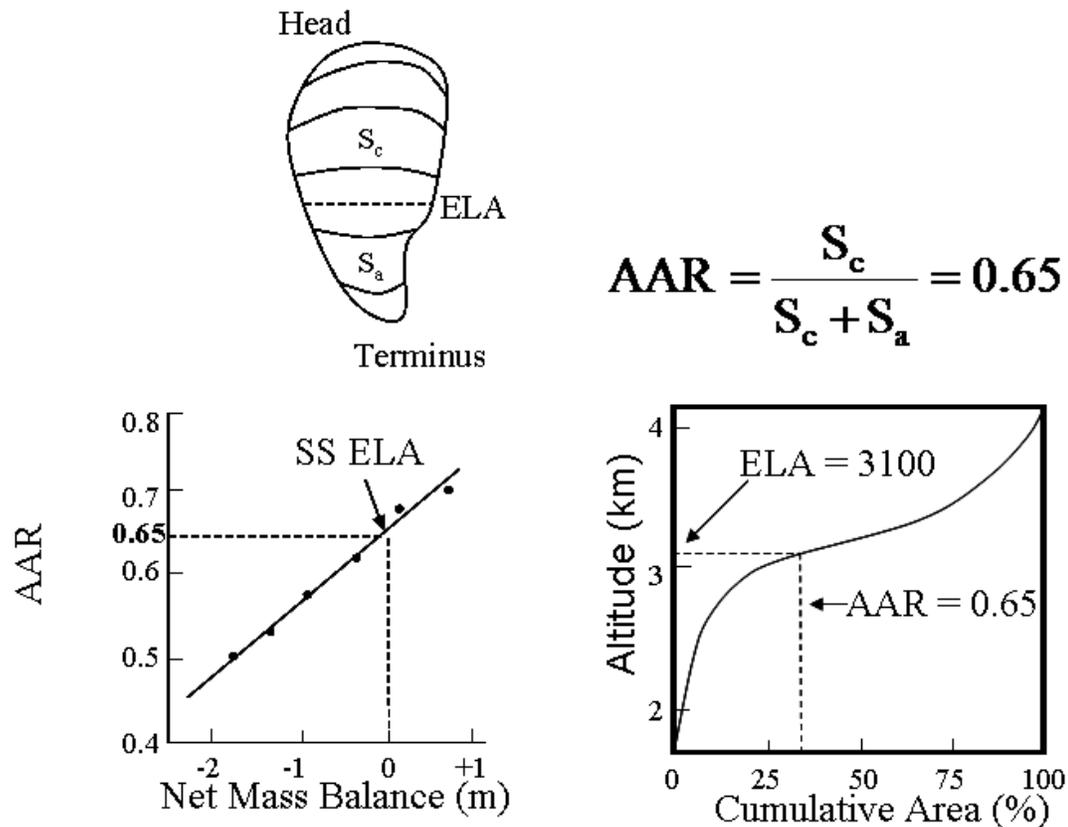
Figure 2.18. Accumulation Area Ratio (AAR). This method is based on the ratio of the accumulation area ( $S_c$ ) to the total area of the glacier, (where  $S_a$  is the ablation area). A steady state (SS) AAR of 0.65 (when mass balance = 0) is regarded as the most appropriate for majority of temperate, debris-free glaciers (Porter, 2001).
