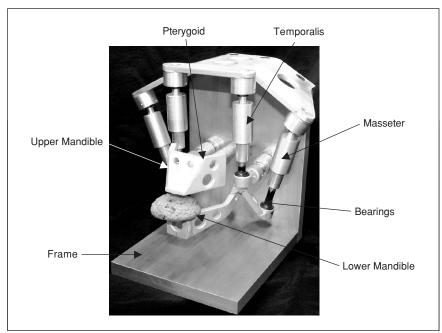
Figure 4. A kinematic model of the robot.
