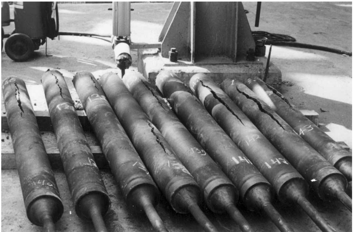
Figure 2: Failed reformer tubes, showing rupture at the lower end where the pigtail exits (Grote & Antonsson, 2008)
