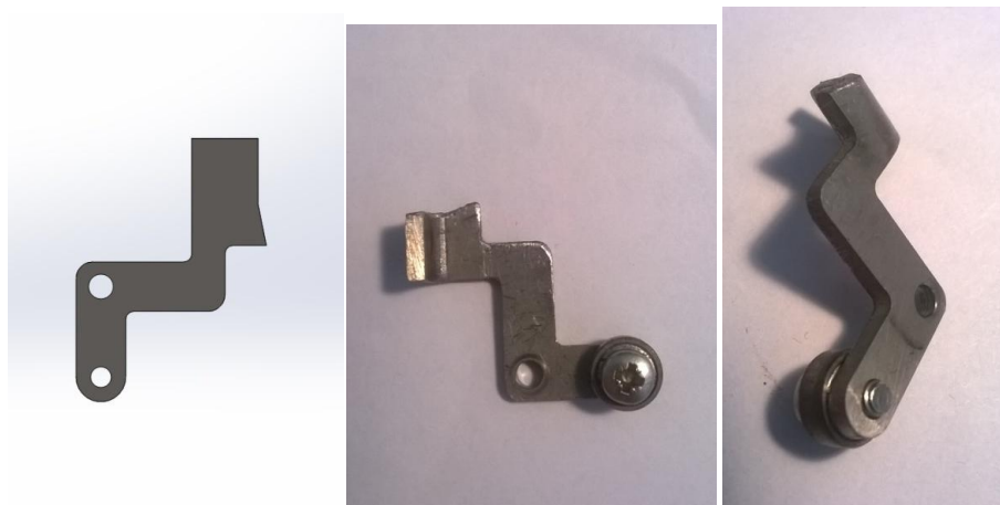
Figure 38: Minimole arm inporvements showing left to right: 3D model; top view, assembled; view of threaded arm connection for bearing.
