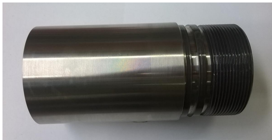
Figure 33: The newly manufactured Upper Economole Spacer
