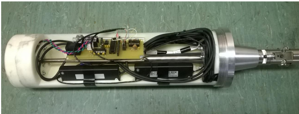
Figure 18: Minimole as received, chassis with cover off
