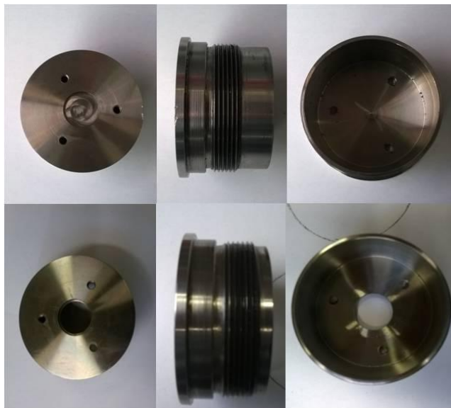
Figure 28: Economole Lower Mount pre modification (top row), and post modification (bottom row)
