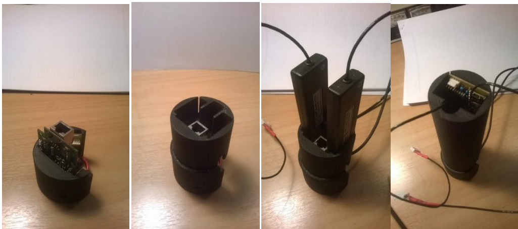
Figure 59: Initial Minimole Electronics Sledge assembly sequence, from left to right
