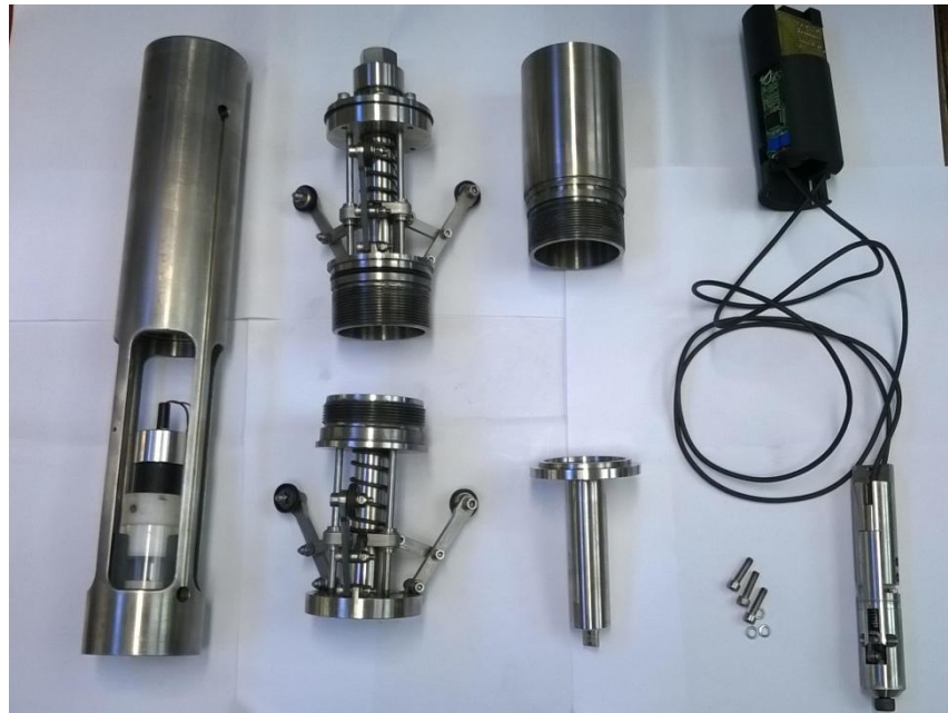
Figure 39: MXmole sub-assemblies (formerly known individually as Economole and Minimole)
