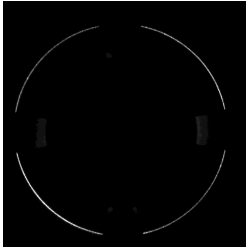
Figure 6: Typical image of ring of reflected laser light seen by the Economole camera
