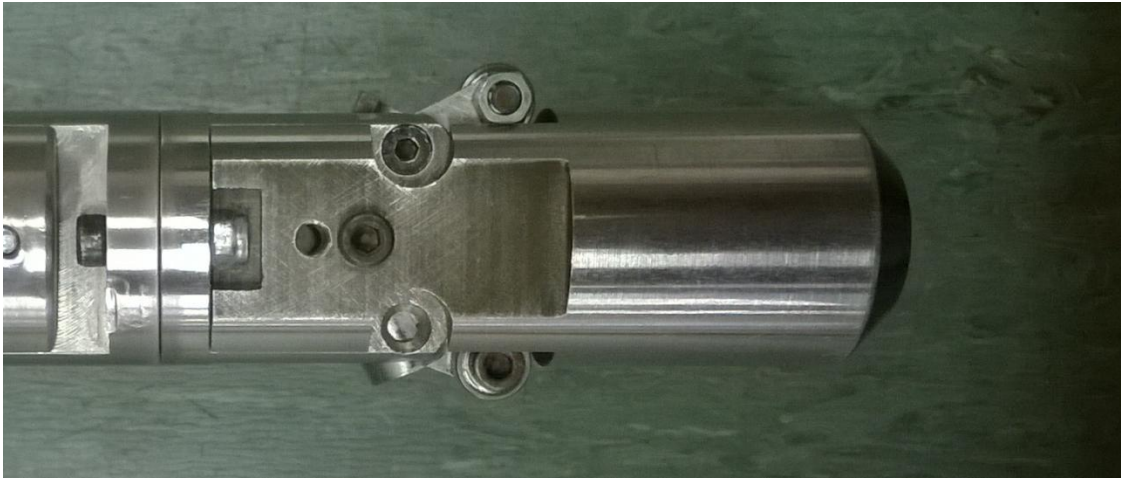
Figure 23: Minimole close up, showing measurement arm assembly
