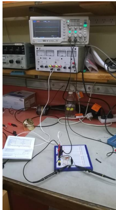
Figure 46: Testing sensor power supply output
