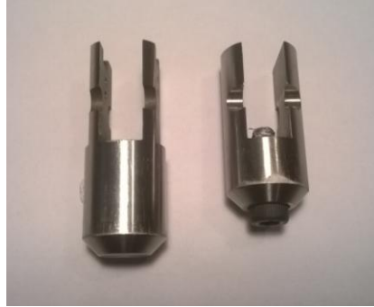
Figure 37: Original Minimole Bottom Case, alongside modified Bottom Case
