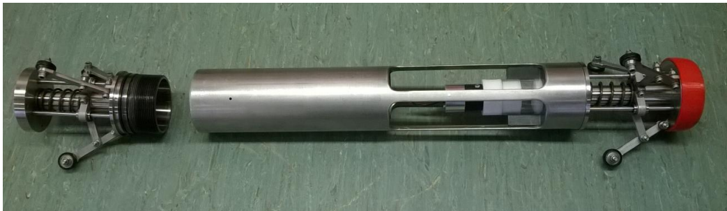
Figure 19: Economole with top wheel-set removed
