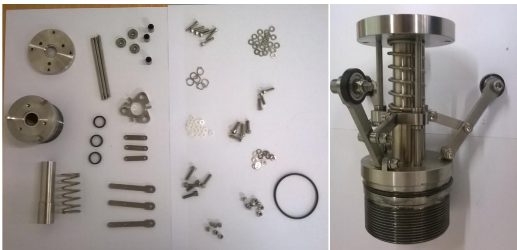
Figure 76: MXmole top wheel-set before and after assembly
