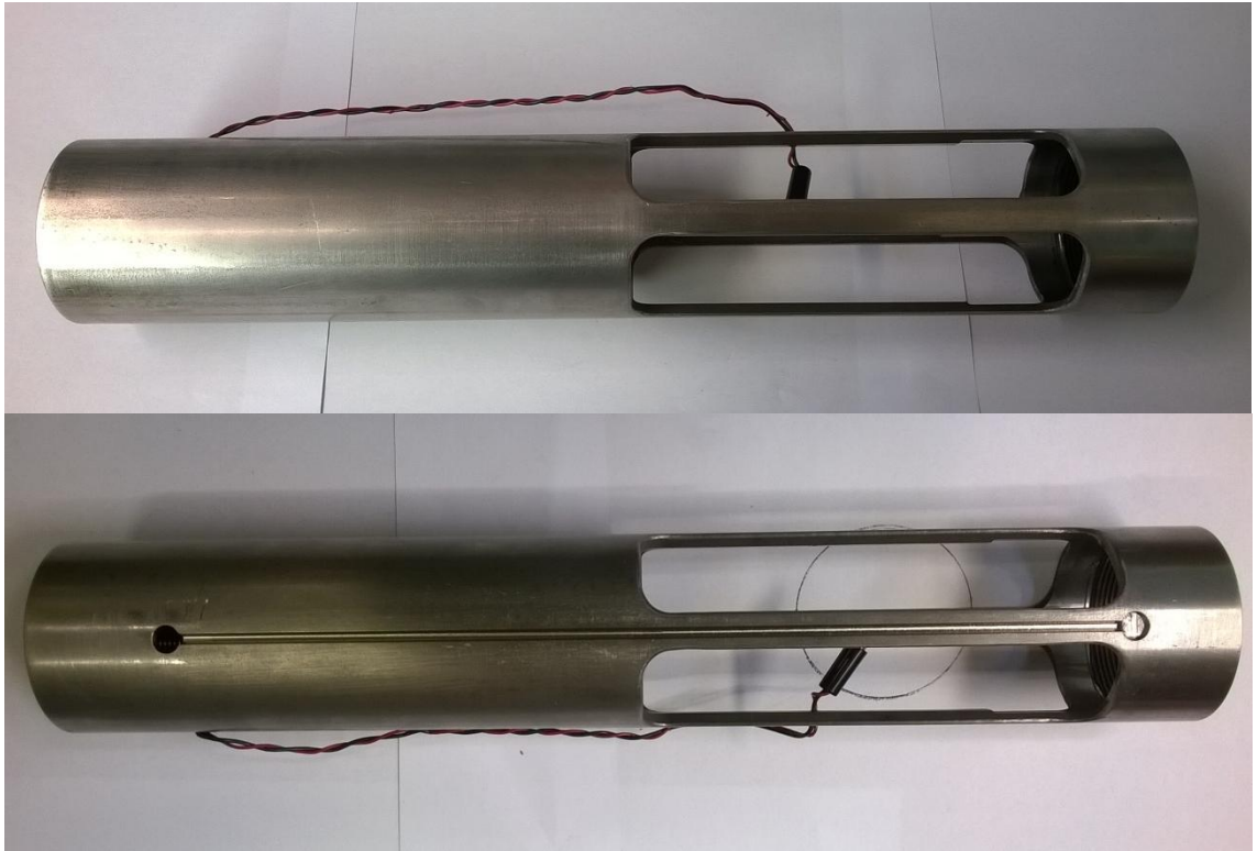
Figure 25: Economole chassis pre and post modification, showing one side with and without one of two sensor grooves and holes
