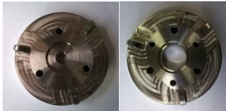
Figure 29: Economole bottom cap pre modification (left), and post modification (right)
