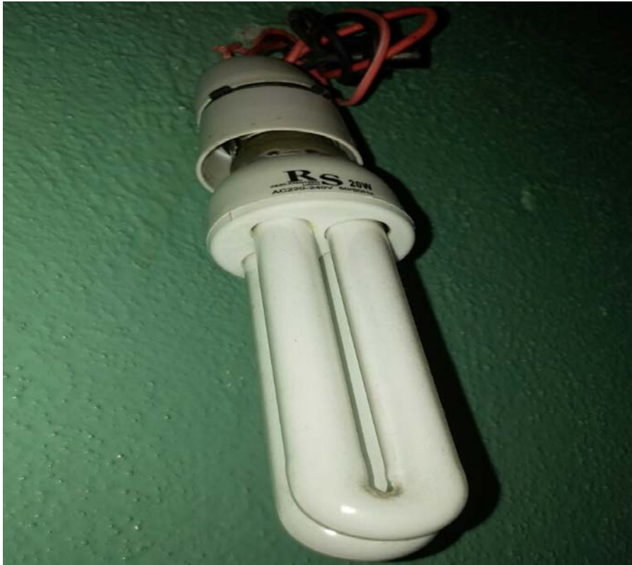
Figure 26: 20W compact fluorescent lamp used in residential dwellings.
