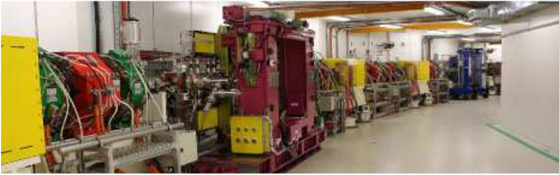
Figure 5-1 Photograph of Australian Synchrotron storage ring, in which electrons travel at close to the speed of light (Australian Synchrotron, 2012).
