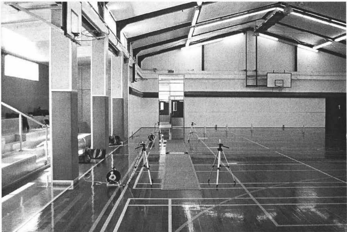
Figure 12 Data Collection Set Up showing the ramp and force plate.
