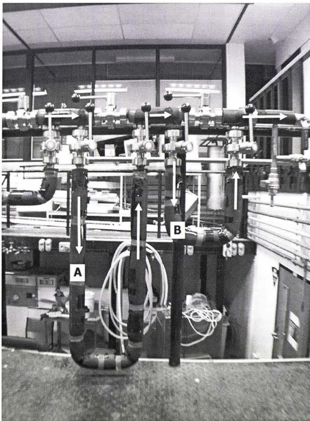
Figure 4.12: Photo of the holding tubes before the evaporator. [A] Holding tube 1, 50 seconds. [B] Holding tube two, 25 seconds.
