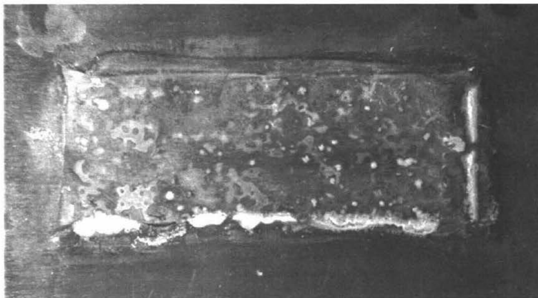
Figure 5.24: Photograph of the plate (Run 35) after the post-caustic rinse. Some fouling can be seen still remaining of the plate after cleaning.
