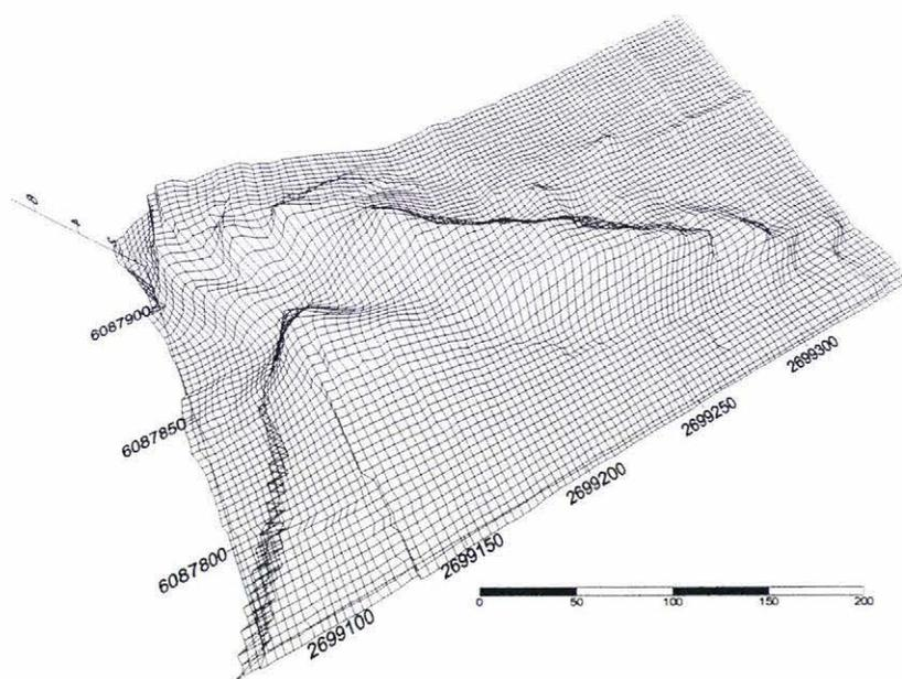
Figure 5.6 Wireframe Map of PD.2 produced using SURFER from data collected by GPS on 7/12/2002. The higher areas represent the depositional lobe, trailing arms and surge lobes.
