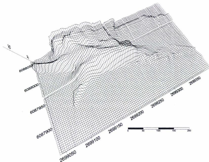
Figure 5.9 Wireframe Map of PD.4 produced using SURFER with data collected by GPS on 8/04/2002. The higher areas represent the depositional lobe, trailing arms and surge lobes.
