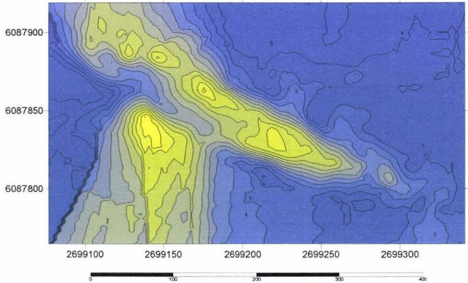
Figure 5.5 Contour Map of PD.3 produced using SURFER from data collected by GPS on 7/12/2002. The high yellow areas are the depositional lobe and trailing arms while the lower surge lobe can be seen extending beyond the depositional lobe and are the greyer areas
