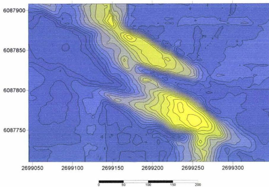
Figure 5.1 Contour Map of PD.2 and PD.3 produced using SURFER from data collected by GPS on 8/04/2002. The high yellow areas are the depositional lobes and trailing arms while the lower surge lobes can be seen extending beyond the depositional lobe and are the greyer areas.
