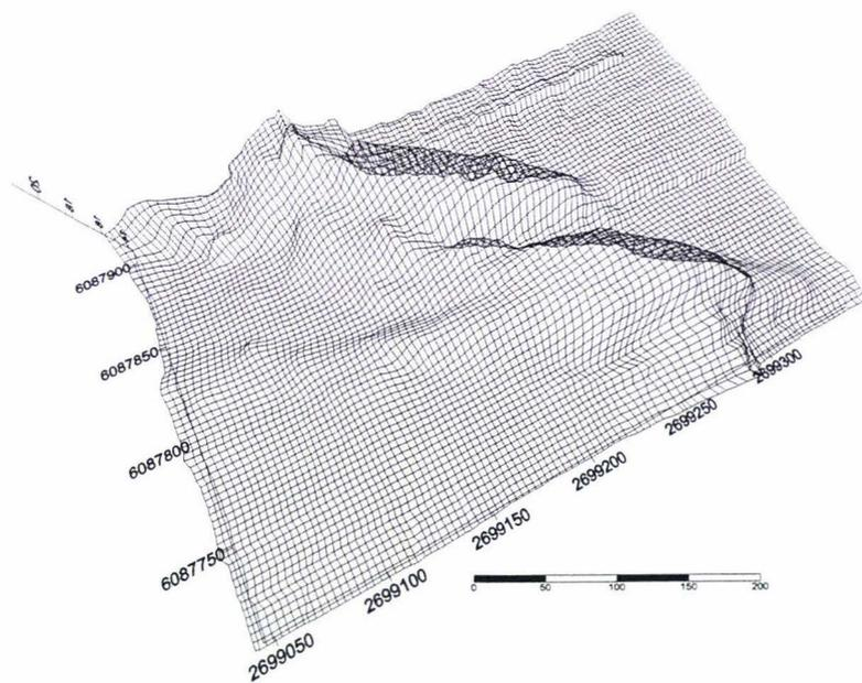
Figure 5.3 Wireframe Map of PD.2 and PD.3 produced using SURFER from data collected by GPS on 8/04/2002. The higher areas represent the depositional lobe, trailing arms and surge lobes.
