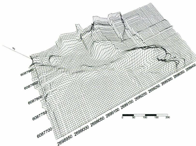
Figure 5.4 Wireframe Map of PD.2 produced using SURFER from data collected by GPS on 7/12/2002. The higher areas represent the depositional lobe, trailing arms and surge lobes. The high region to the left of the depositional lobe is unrelated to PD.2.
