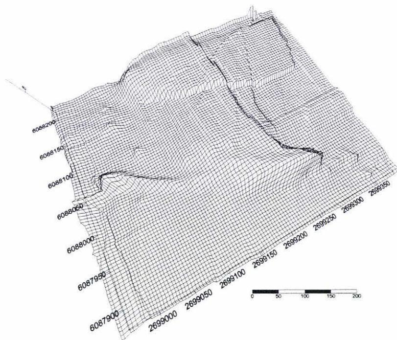
Figure 5.10 Wireframe Map of PD.4 produced using SURFER with data collected by GPS on 7/12/2002. The higher areas represent the depositional lobe, trailing arms and surge lobes.
