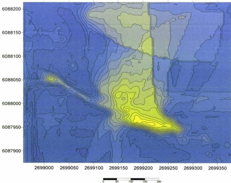
Figure 5.8 Contour Map of PD.4 produced using SURFER with data collected by GPS on 7/12/2002. The high yellow areas are the depositional lobe and trailing arms
