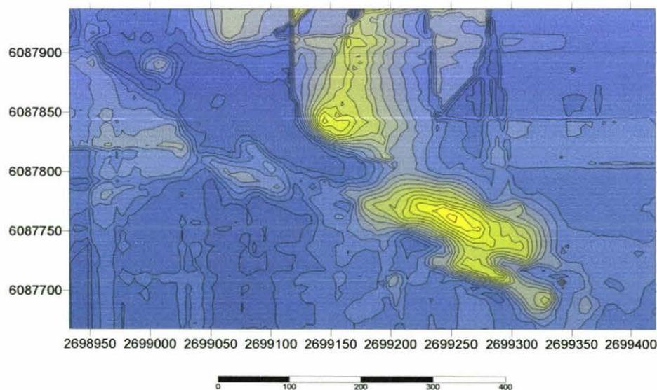
Figure 5.2 Contour Map of PD.2 produced using SURFER from data collected by GPS on 7/12/2002. The high yellow areas are the depositional lobe and trailing arms while the lower surge lobe can be seen extending beyond the depositional lobe and are the greyer areas.
