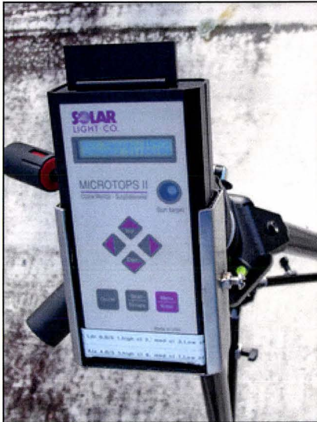
Figure 2.2: View of MICROTOPS instrument (top) and operation on the roof of Land-care building (bottom).
