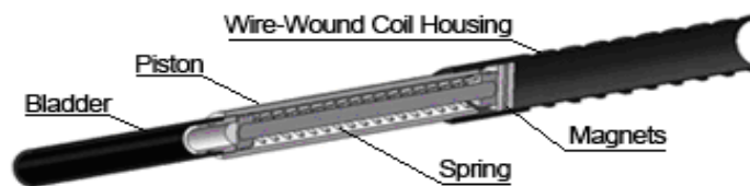
Figure 5: CAD model for proposed electromagnetic energy harvester
