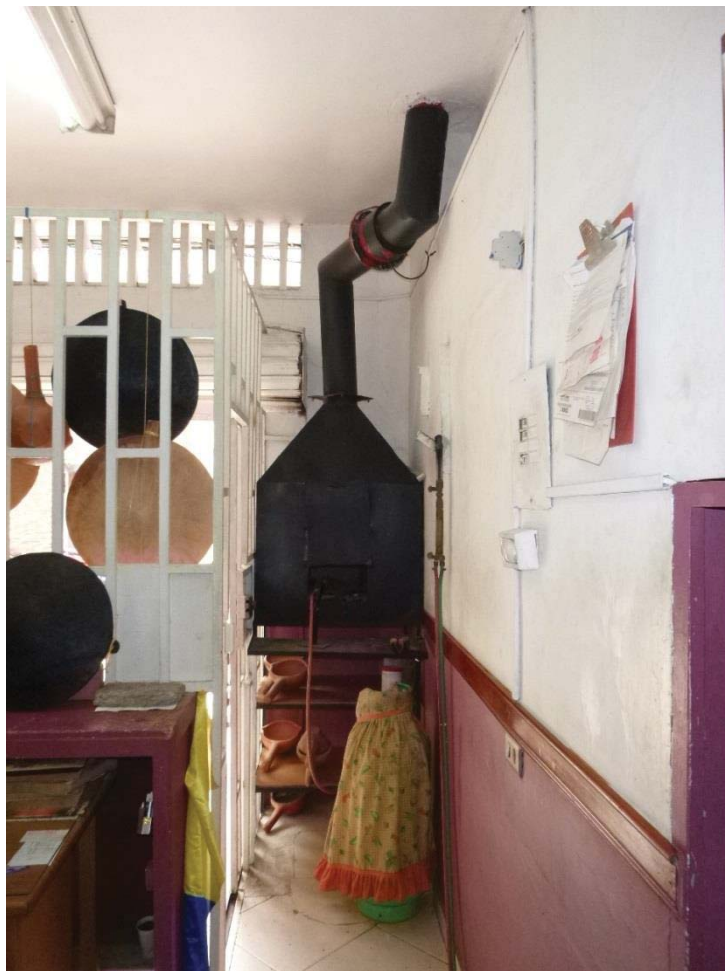
Figure 13: The fume hood where the amalgam is burned.
