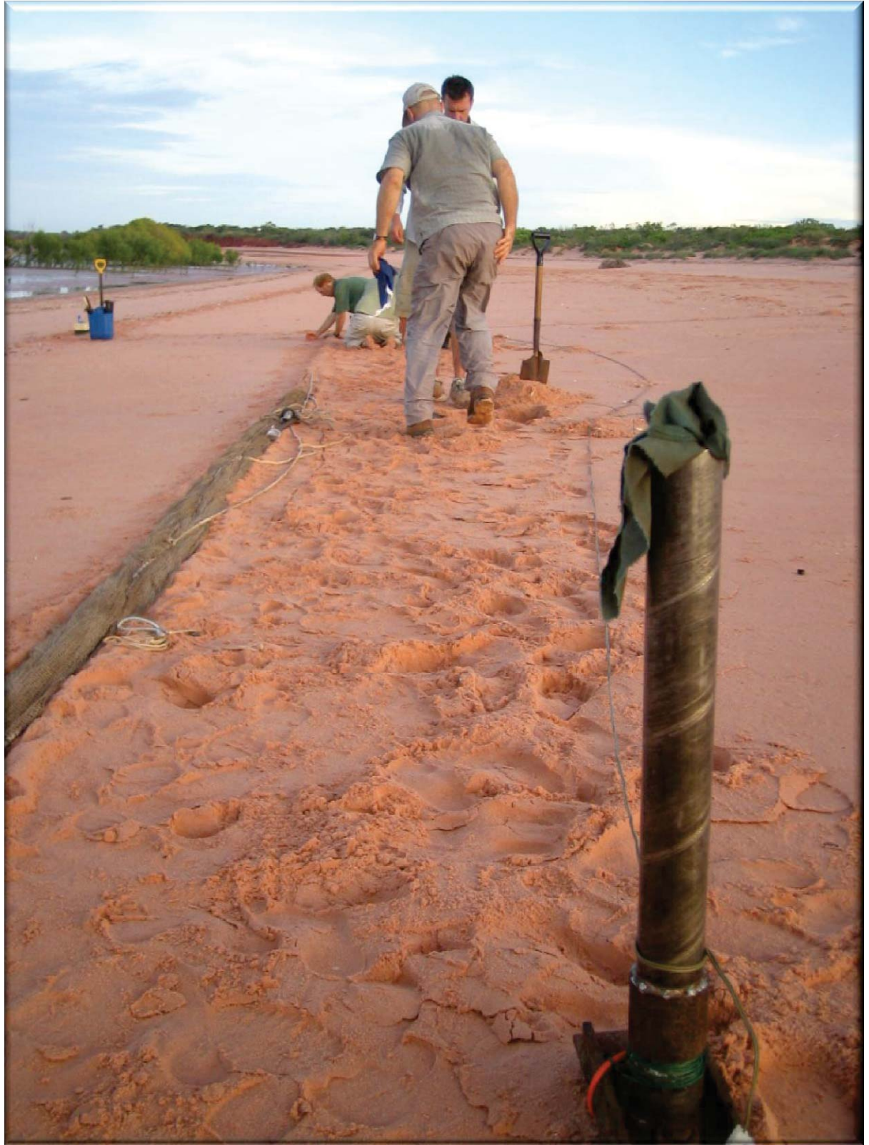
Figure 2. A cannot-net is prepared for firing. This involves camouflaging a mesh net behind where the birds are expected to roost. Cannons, like the one shown here, are partially buried in the sand. Projectiles are tied to the leading edge of the net. A
