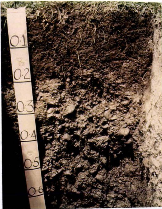
Figure 2.4 b) A typical profile of the otukura stony silt loam, mottled phase (site shown above). Note the 20cm of brownish black silt loam Ap horizon over a very stony ABg horizon. Below this, at 35-50cm depth is a gleyed, mottled stony Bgm horizon. At 50-75cm depth the profile has prominent bright brown mottles in a very gleyed sandy matrix.
