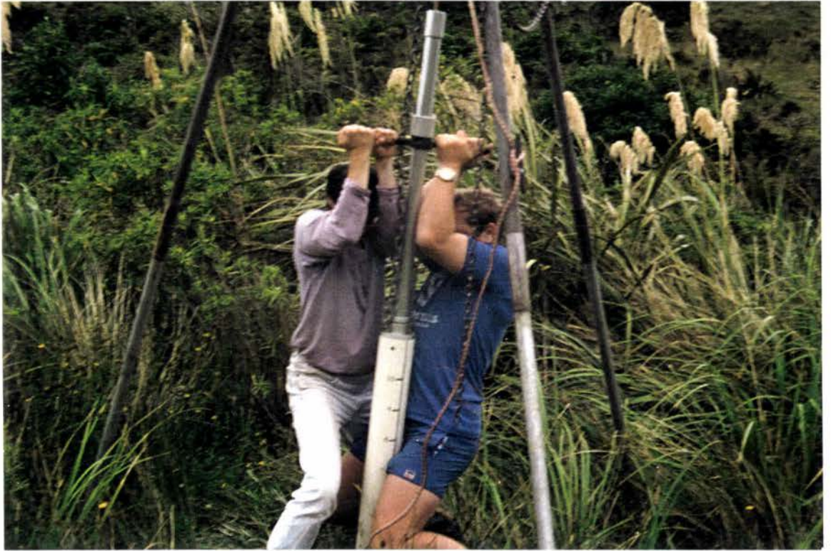
Figure 3.4 The Neale corer being used to core compacted sediments at Kashmir
