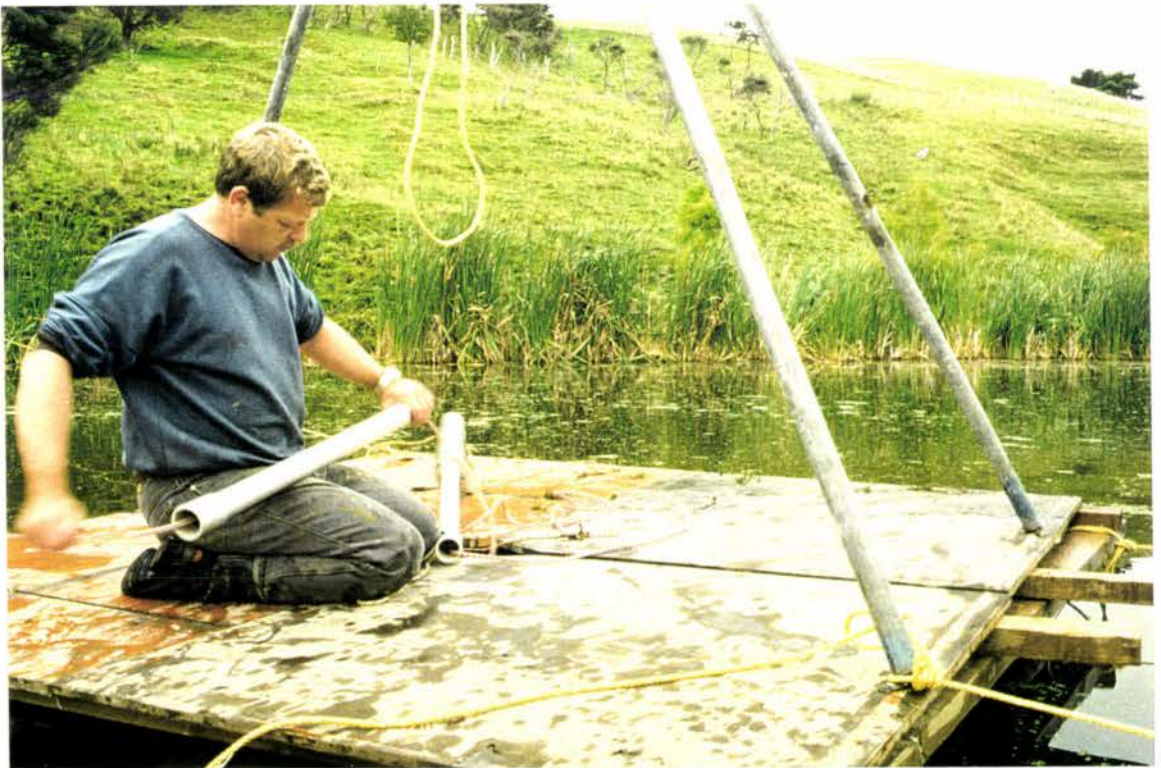
Figure 3.3 Preparing the Neale corer for use from the raft at a deep water site at Big Hill
