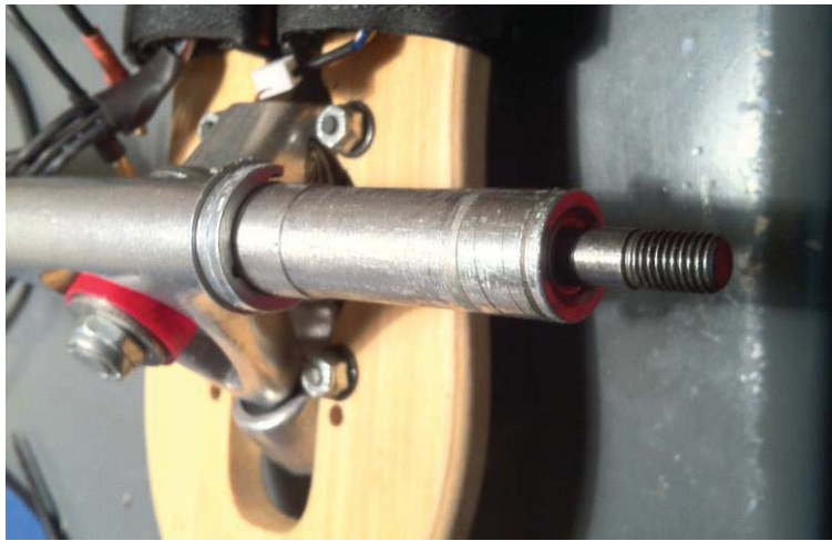
Figure 3.9 - The longboard truck after machining, extension of the aluminium axle, and location of the inside end bearing mount.
