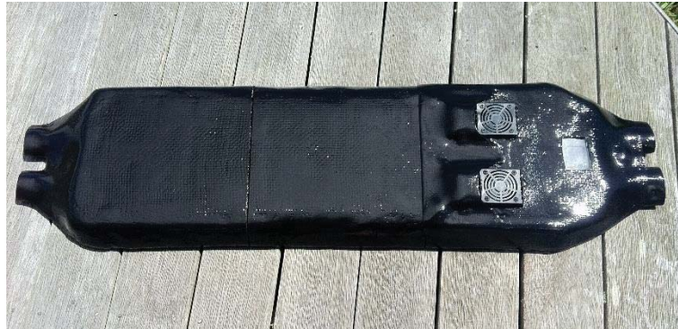
Figure 3.16 - Fibreglass enclosure for the electrical components of the electric longboard.
