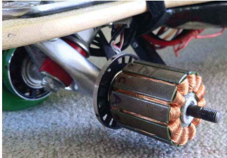
Figure 3.10 – Photograph of the modified longboard truck and stator assembly.
