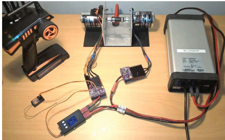
Figure 5.1 - Test rig used for the bench testing of the motor controller and the comparison of the two motor control techniques.
