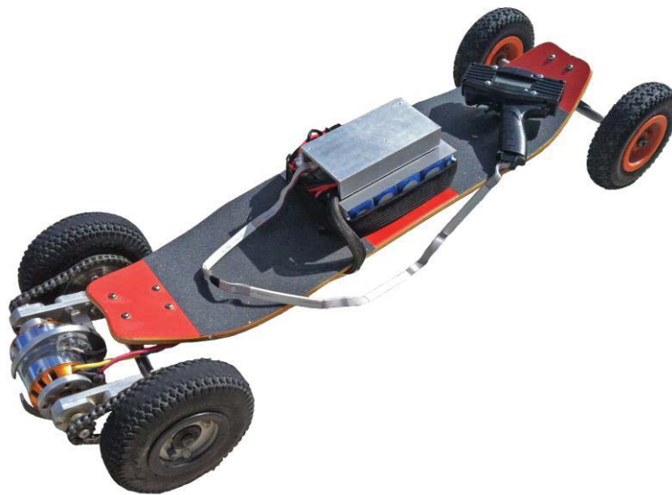
Figure 3.1 - Electric mountain board prototype built as part of final year engineering project.
