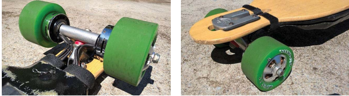
Figure 3.15 - Photograph of the actual electric skateboard hub motor assembly viewed from the underside (left) and the top side (right).
