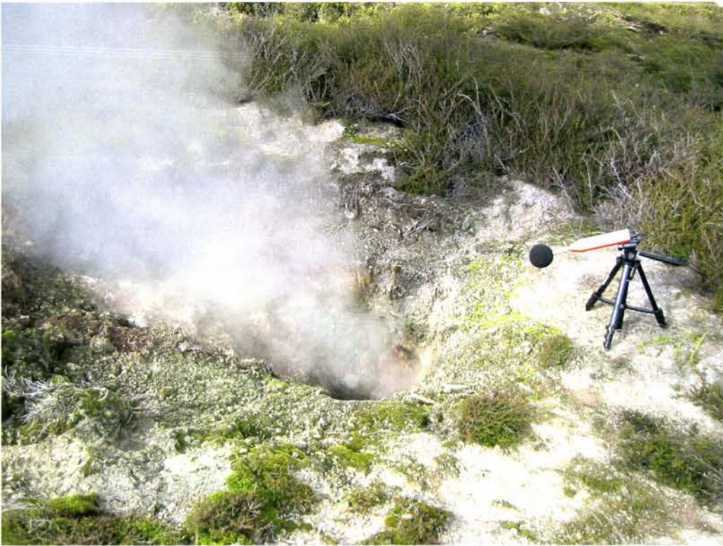
Figure 5.3: A fumarole's sound being measured by a sound level meter
