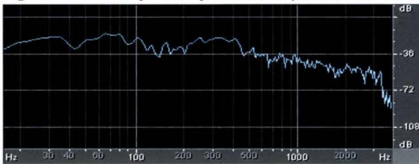
Figure 5.15: Spectrum analysis of mud bubble collapse sound at 0.6 second
