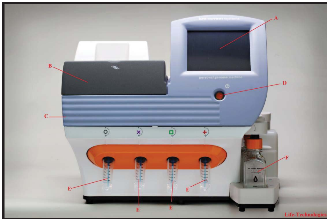
Figure 6 – Ion-Torrent PGM sequencer, A) touch screen control, B) Ion-chip loading deck clamping mechanism, C) special material grounding plate, D) power button, E) Reagent bottles, F) Wash bottles.
