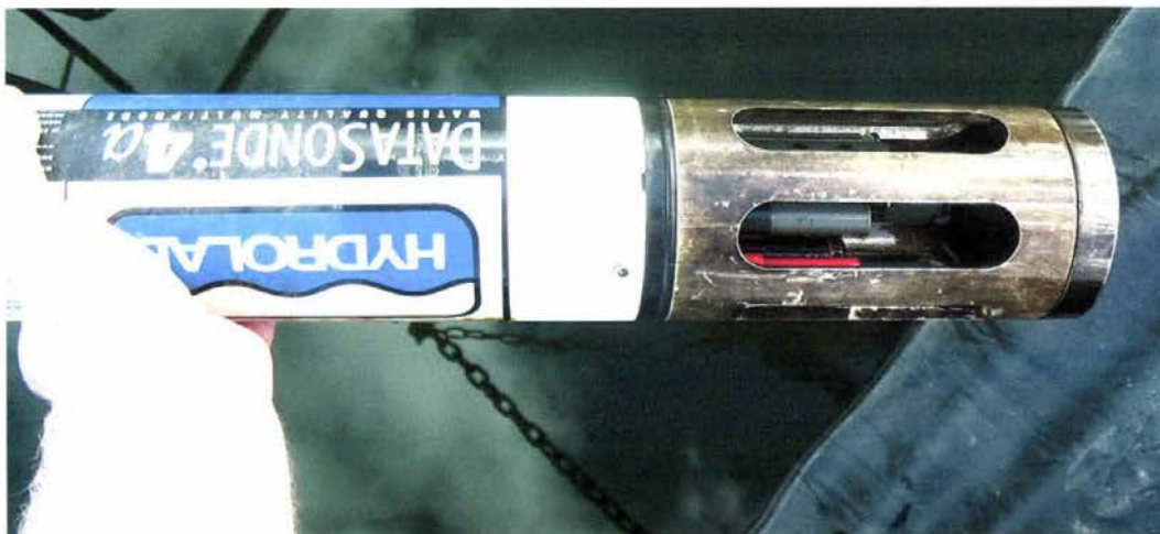
Figure 2.9: Close-up of a Hydrolab datasonde 4a, deployed in one of the pilot-scale HRAP at Ruakura. The individual probes are protected by a solid guard.
