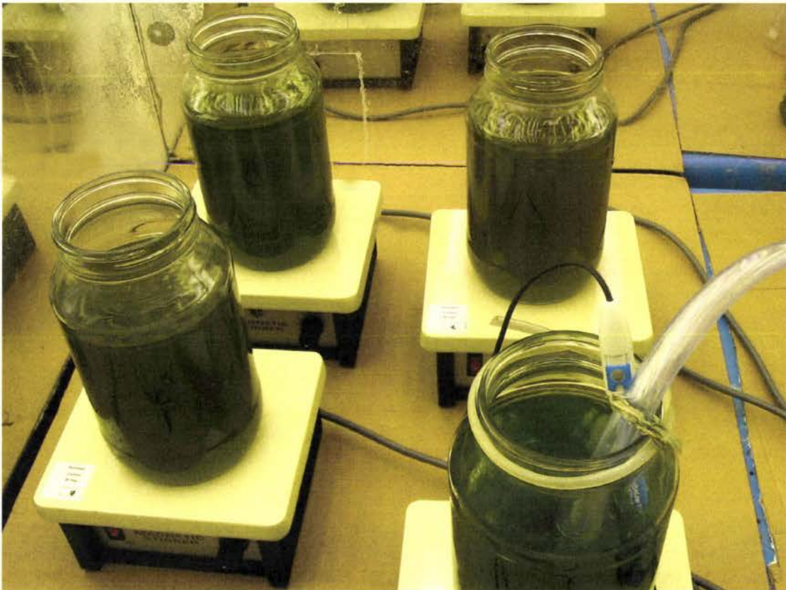
Figure 2.2: Laboratory batch experiment with one algal culture microcosm with CO 2 addition (front right) and three control algal culture microcosms, grown under constant conditions.
