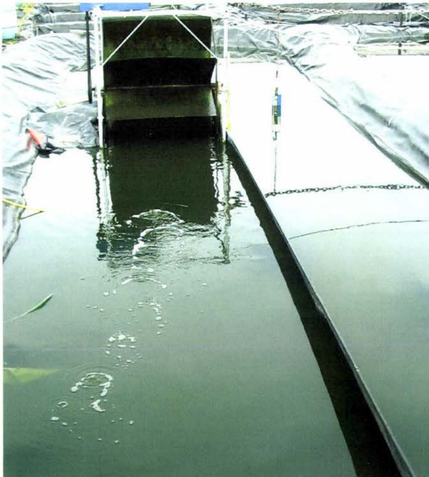
Figure 2.8: Carbon dioxide addition to the eastern HRAP close to the paddlewheel, where water column turbulence is greatest.
