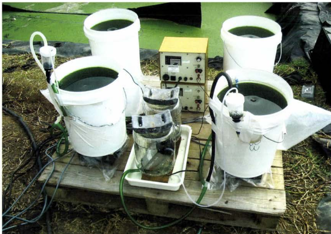
Figure 2.4: Outside mesocosm experimental setup showing four algal culture mesocosms, two with pH controllers and CO 2 addition (front) and two control cultures without CO 2 addition (back).
