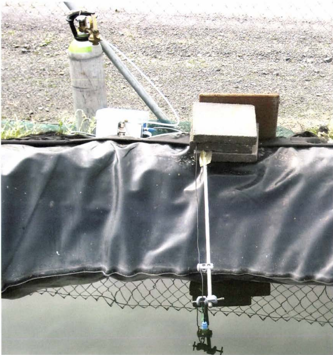
Figure 2.6: High rate algal pond pH controller and CO 2 gas bottle.
