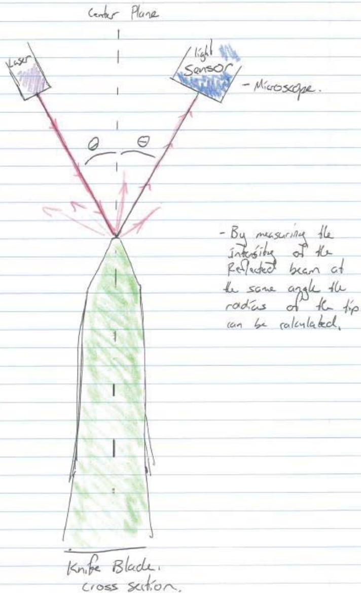
Figure 25: Laser light reflecting concept.
