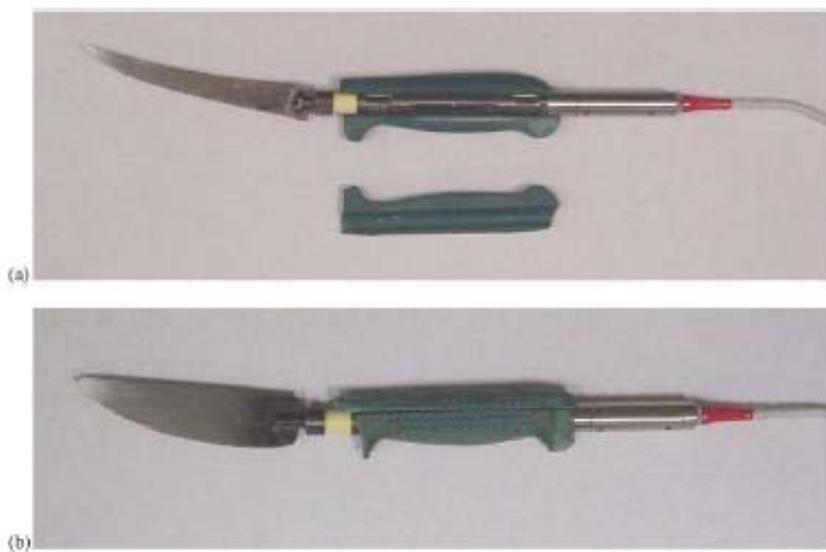
Figure 3: McGorry (2005), grip force knife handle, (a) boning knife, (b) skinning blade.
