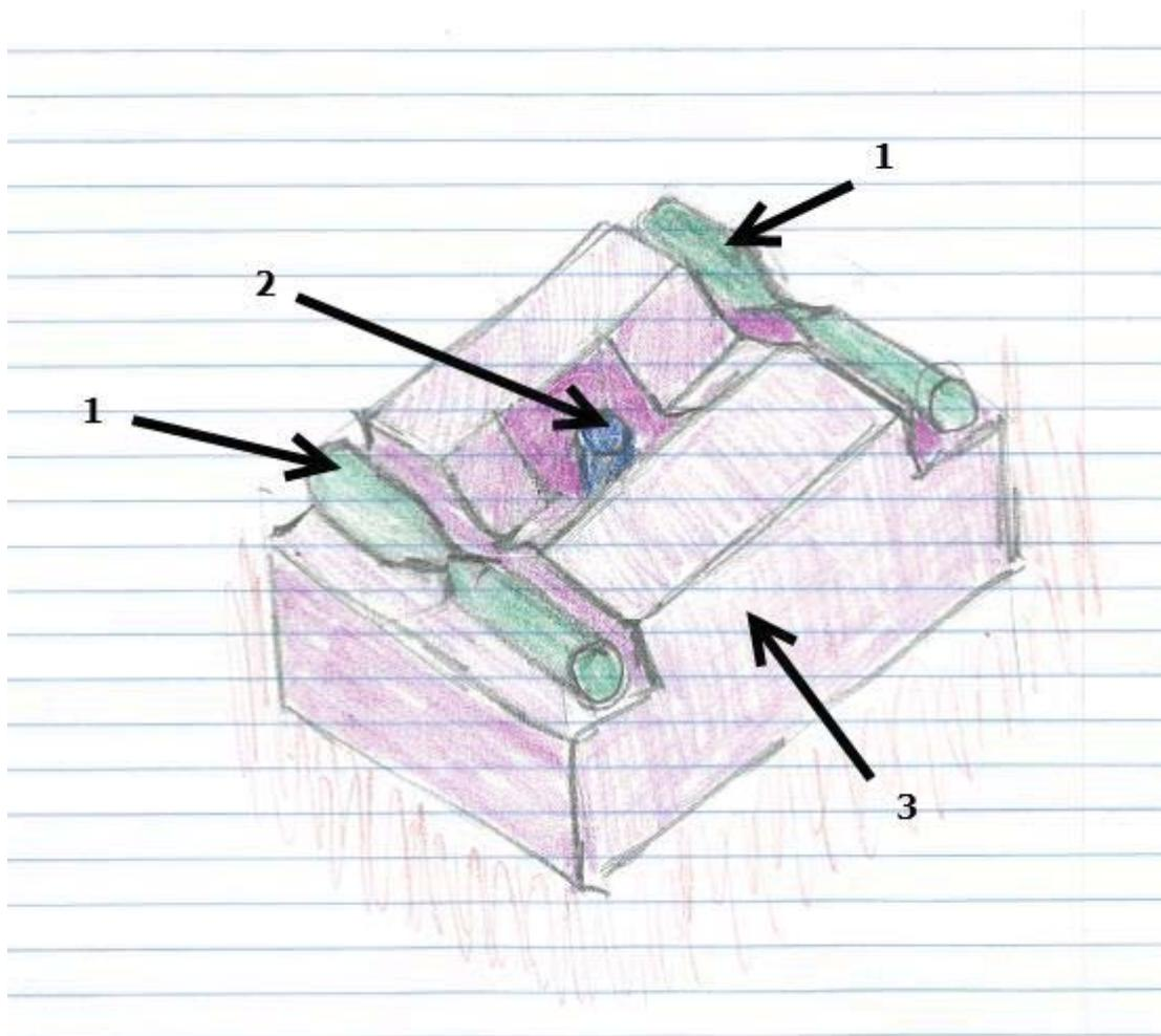
*Figure 12: First concept of Capacitance probe test rig. 1 – Roller guides, 2 – Capacitance probe sensor, 3 – test rig frame.*
