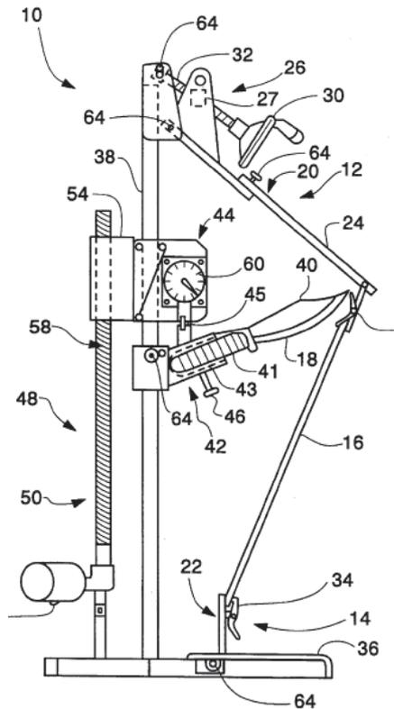
Figure 7: US5571956 (1996) knife sharpness testing machine, 60 – load cell, 16 – test material, 50 – drive motor, 30 – material tensioner.
