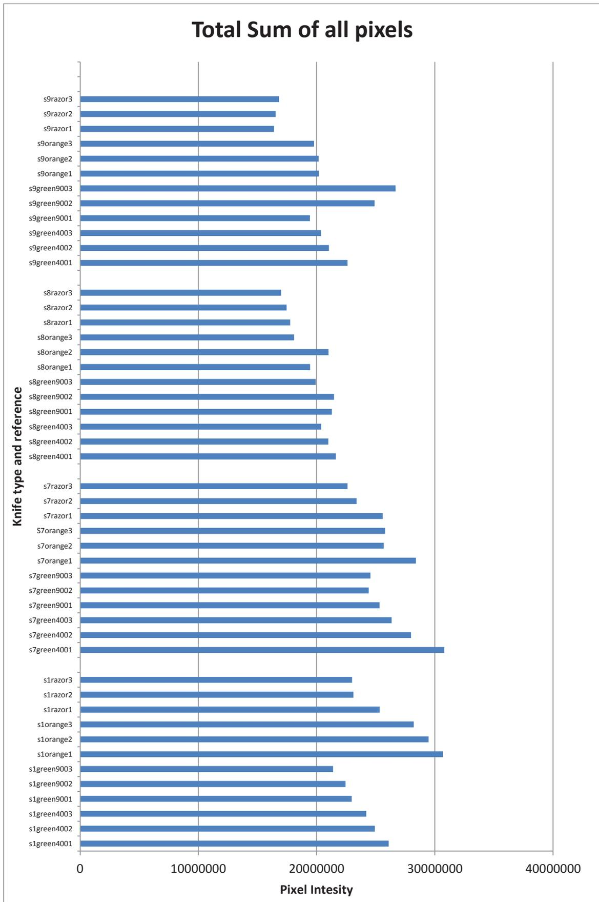
Figure 24: Total sum of the brightness of the reflected laser light.
