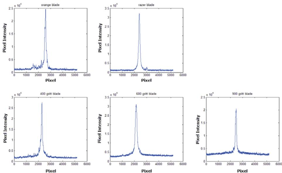
Figure 21: Normal distribution of pixel values of the columns summed.
