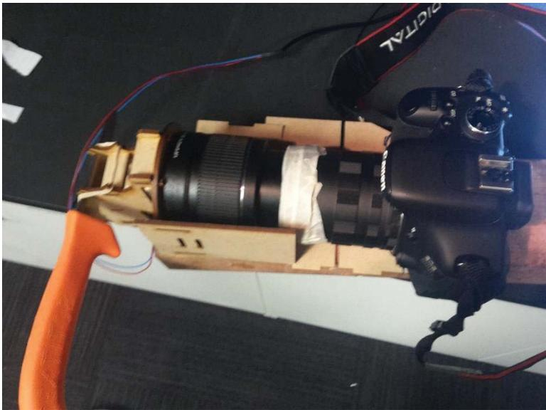
*Figure 15: Test rig for laser reflection experiment. (Top)*
