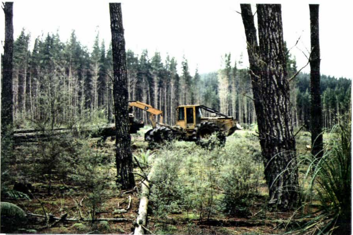
Figure 7: Grapple Skidder Extracting Felled and Delimbed Stems From The Cutover.
