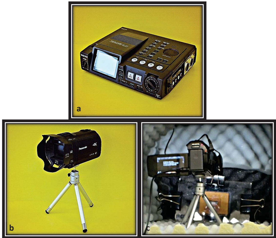
Figure 2.7: Recording instruments used for the experiment; a) sound recorder (TASCAM DR-05, Linear PCM Recorder), b) video camera (Panasonic High Definition-4K Video Camera, Model No: HC-VX870M), c) camera set-up in front of the cambium sandwich.
