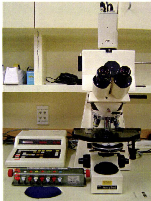
Figure 2.6. The Zeiss microscope and counter used for scoring the micronucleus assay. The counter is displayed on the left side of the picture and was used to keep a running total of the numbers of binucleate cells with each number of micronuclei.
