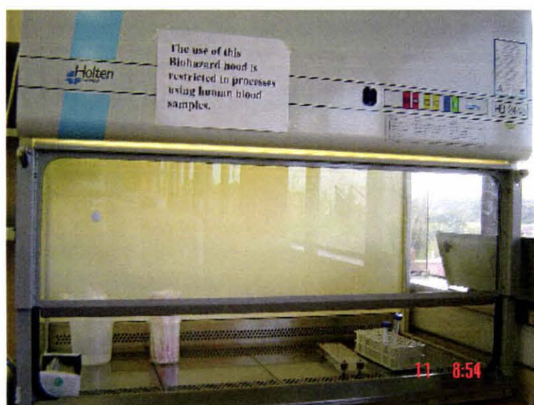
Figure 2.1. A photograph of the Biohazard Hood used for all blood manipulations to avoid contamination. The system can be sealed off by the UV light unit which sterilises the surface.
