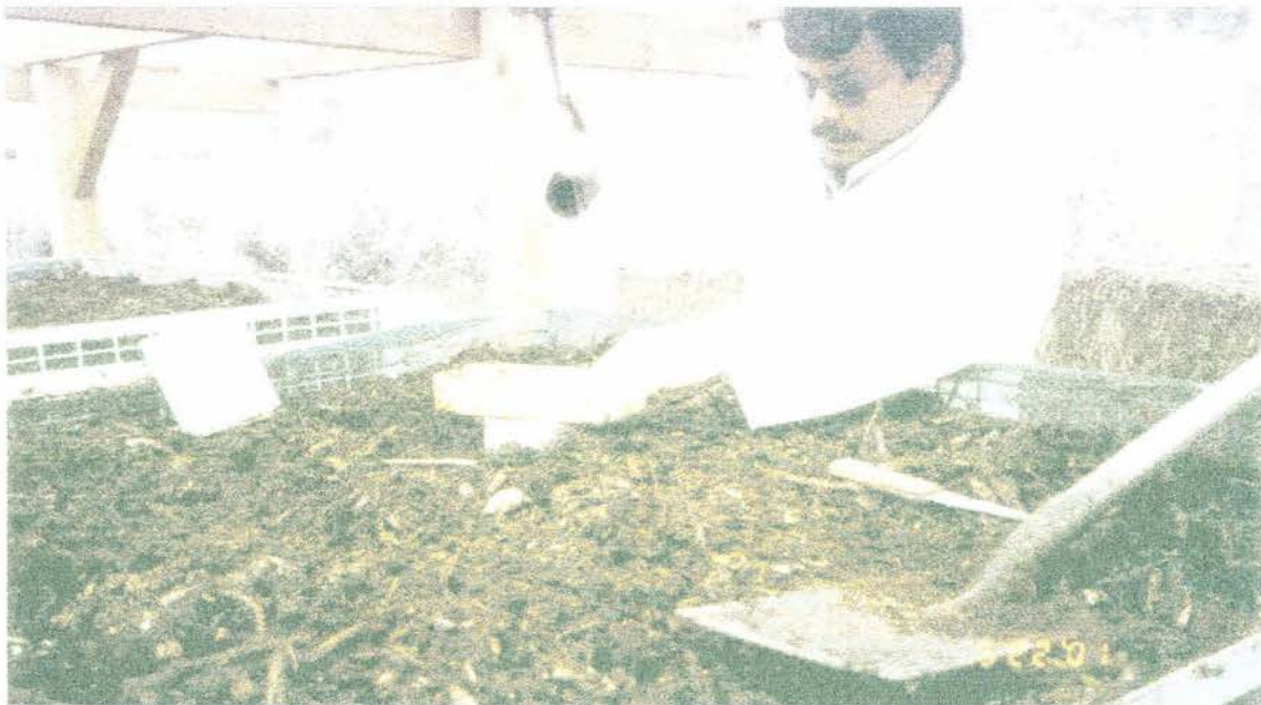
Fig. 4.10 The core cutter is hammered in to collect sample for bulk weight.
