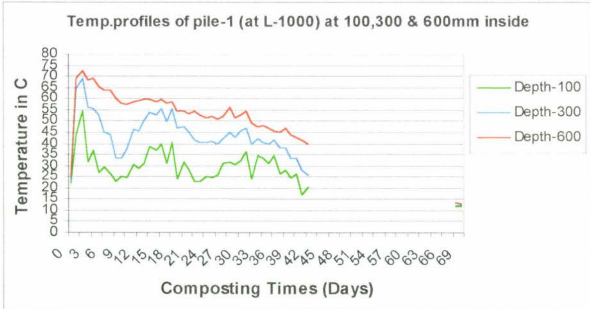
Fig.J.4 Temperature profiles (pile-1 of Experiment-I) at 100, 300 & 600mm inside from front edge of pile (at Level-1000mm above pile base).
