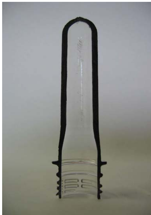
Figure 3-1: Section of the Visy preform (29gr. pure PET)
