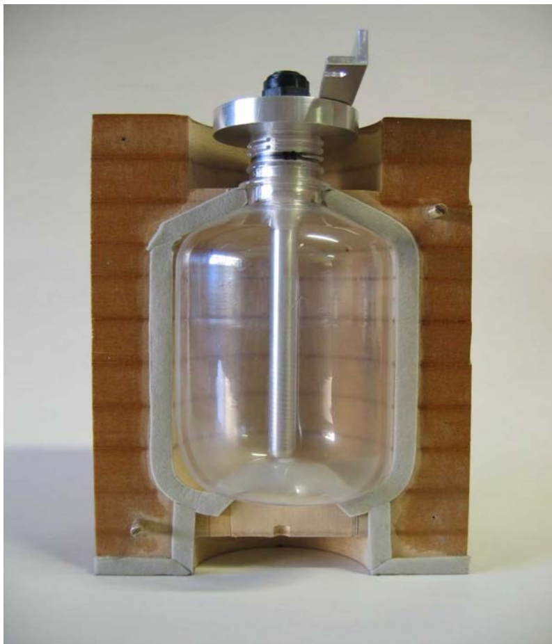
Figure 4-11: Mould half with blown bottle and aluminium rod in place
