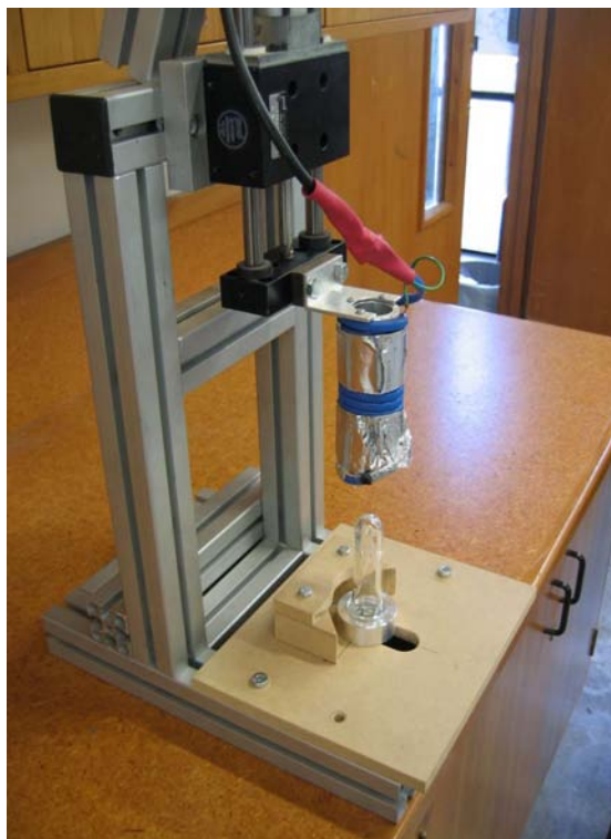
Figure 4-2: Aluminium heating tube installed on a linear guides
