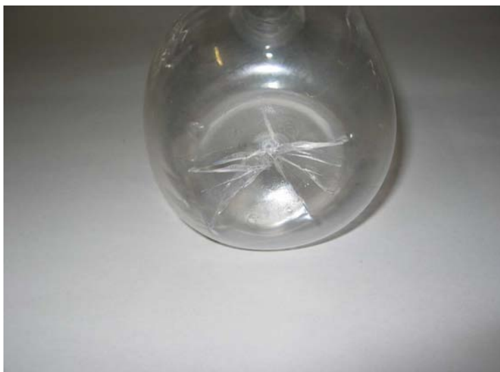
Figure 4-12: Detail of a bottle after burst pressure testing
