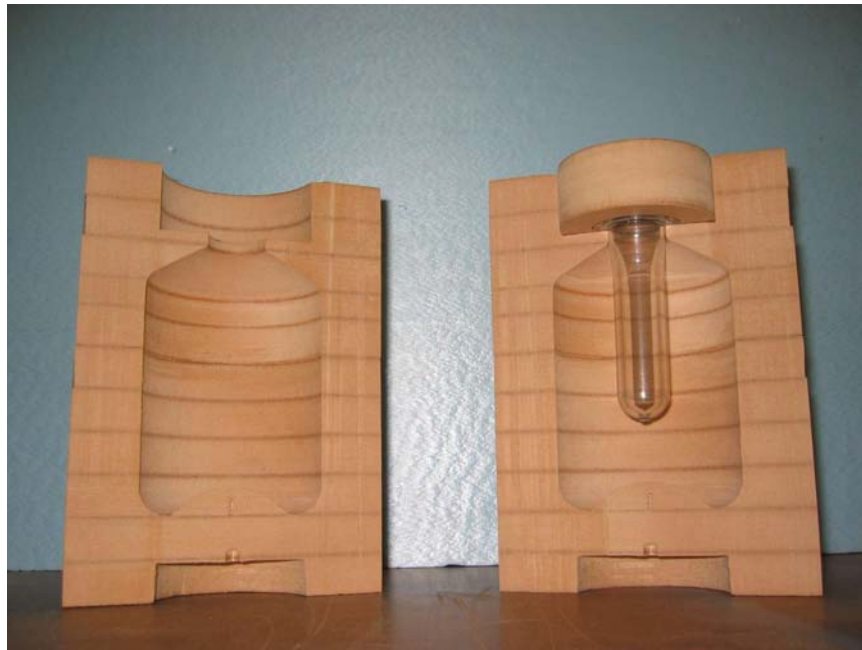
Figure 4-7: Split wooden mould halves with preform in place
