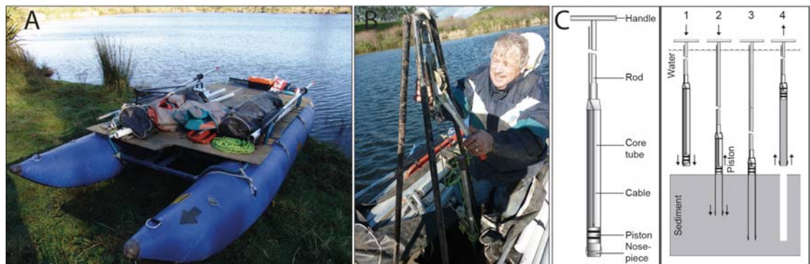
Figure 2. 2 (A) Shows the raft and the equipment used for coring the lake sediments. (B) Illustrates the jack, which was required to lift Livingston piston-corer from the lake bottom with technician David Feek. The lake shown in both images is Lake Richmond, which was first cored during this study. (C) Diagram from Woodward and Sloss (2013) showing the piston corer components similar to that used during this study, and its coring operation with (1) the corer positioned above the sediment surface and (2-3) subsequently pushed into the soft sediments, while simultaneously keeping the core-cable tight so as to create suction until the desired depth has been penetrated, (4) the corer extracted with the sediments.
