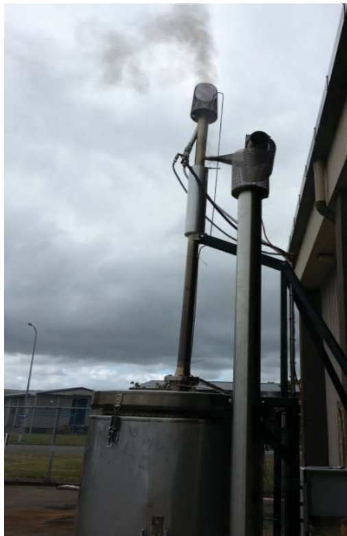
Figure 2-1: Batch pyrolysis reactor designed and built by Bridges (2013) during a run with 70 kg of wood chips.
