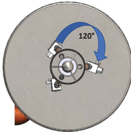
Figure 2-5: Plan view of the flare showing the angle of the burners, arranged in a triangular pattern around the flue stack
