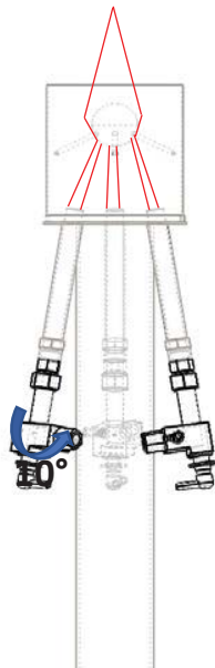
Figure 2-6: Elevation view of the flare showing the angle of burners relative to flue stack
