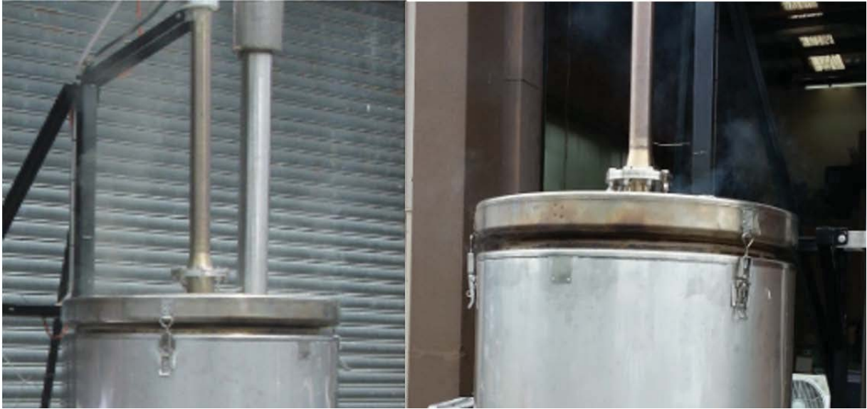
Figure 2-8: Fugitive emissions seen during a pyrolysis run with 70 kg of wood chips
