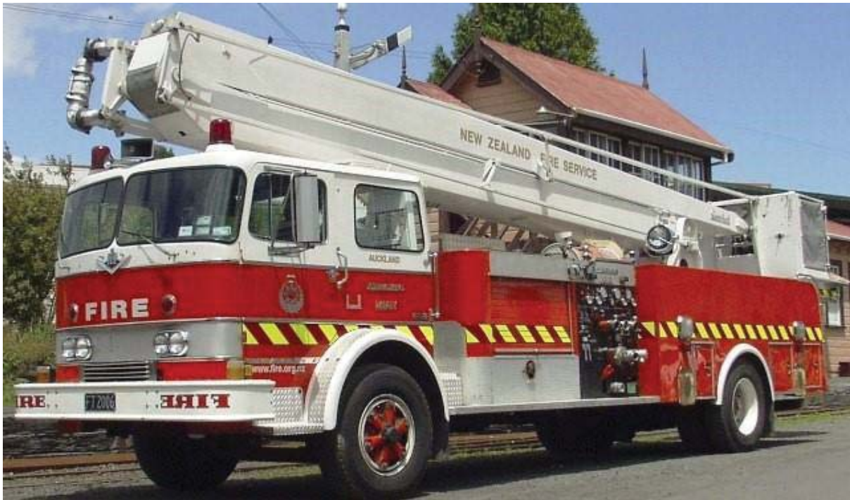
Figure 4. 1971 Darley International Snorkel (Type 5) fire appliance. Photo courtesy of The Museum of Transport and Technology (MOTAT).
