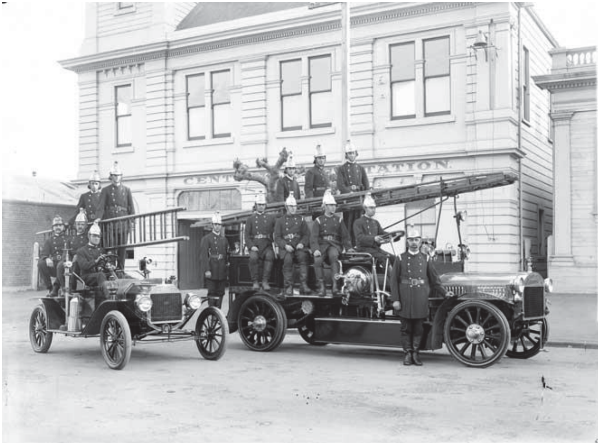
Figure 3. Members of the Whanganui fire brigade pose with their Merryweather fire engine (right) and a modified Model T Ford, in 1919. Used with permission of the Alexander Turnbull Library, F. J. Denton Collection. Reference: 1/1-020869; F. Photograph by Frank J. Denton
