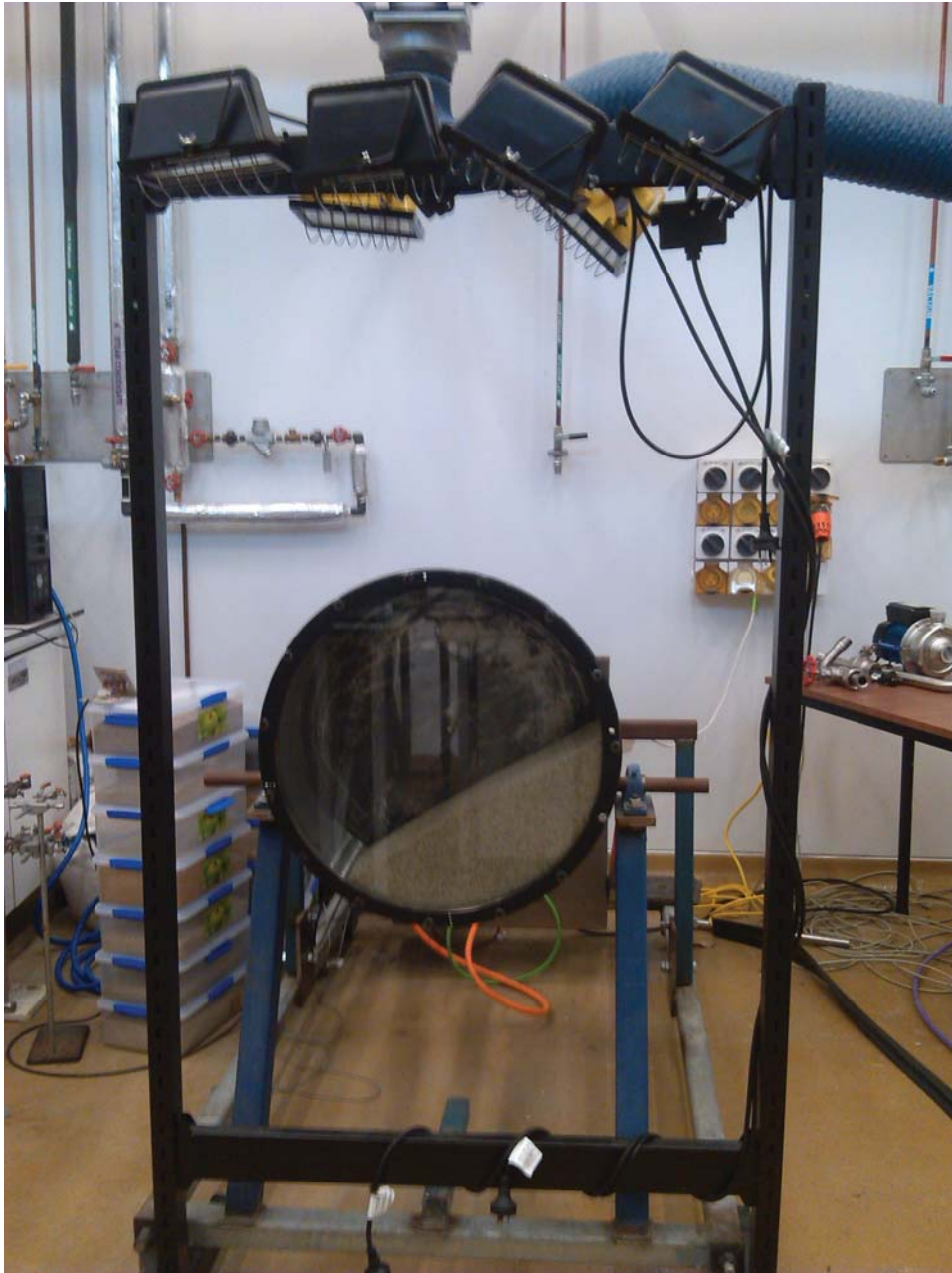
Figure 3.2.1: The lighting rig constructed for this research. There are four 500W halogen lamps mounted on a custom frame, constructed from spare office shelf mounts. The two lamps mounted to the reverse of the rig were not used. On the left of the image, just visible is the computer used to control the drum motor, and the stack of airtight boxes used to store samples. Photograph taken by the author.
