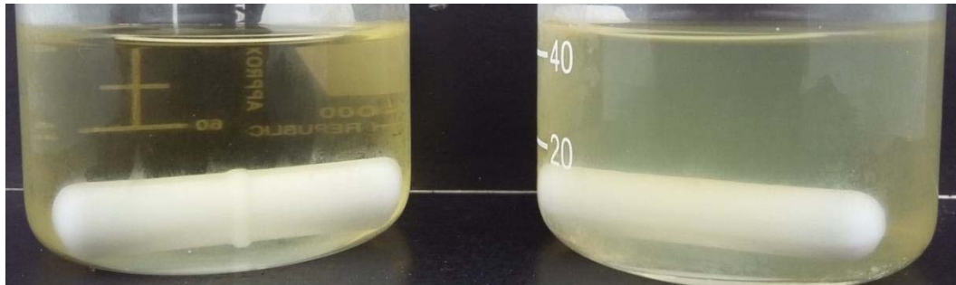
Figure 6-15: Acid clarified cow (left) and goat (right) caseinate digests after ferrous sulfate addition of 90 mM final concentration.
