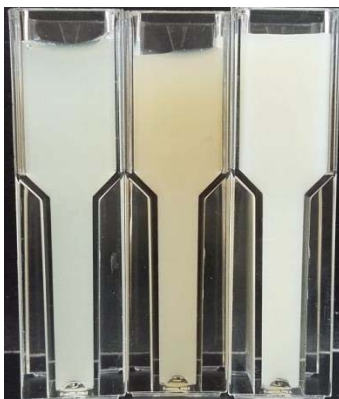
Figure 5-9c: Cow caseinate (3.0 %) fortified with 5 mM, 11 mM and 22 mM ferrous sulfate with an adjusted pH to 6.7 after fortification.
