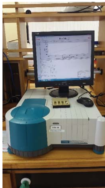
Figure 7.2 – UV Spectrophotometer device used in this experiment.
