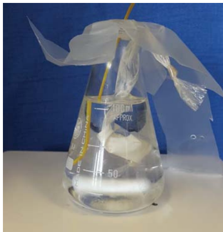
Figure 7.7 – Parafilm used to seal the container and prevent evaporation of the water in the container.
