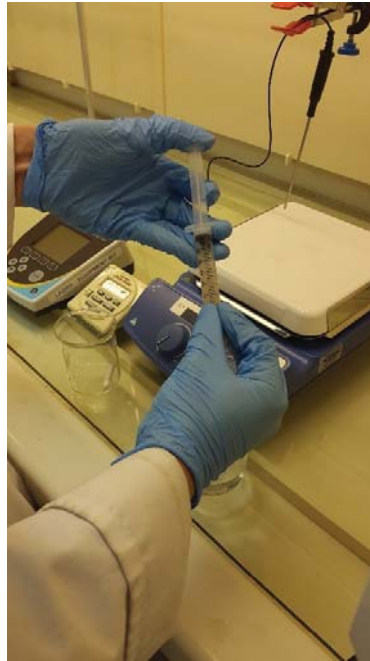
Figure 7.4 – Injection of the sample into the dialysis membrane.
