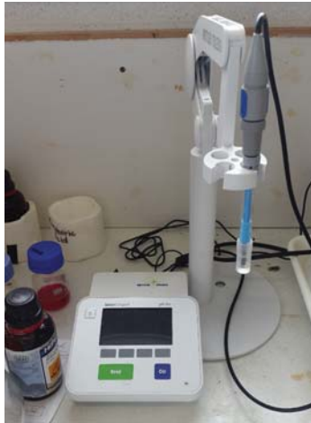
Figure 7.12 – The pH meter used to adjust the pH on 4.9 for mobile phase preparation.
