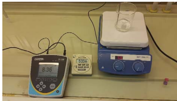
Figure 7.5 – pH and temperature meter on the left, the timer in the middle and the hot plate in the right corner. The beaker is on the hot plate, and the detector is inside the beaker for detecting the temperature of the solution.
