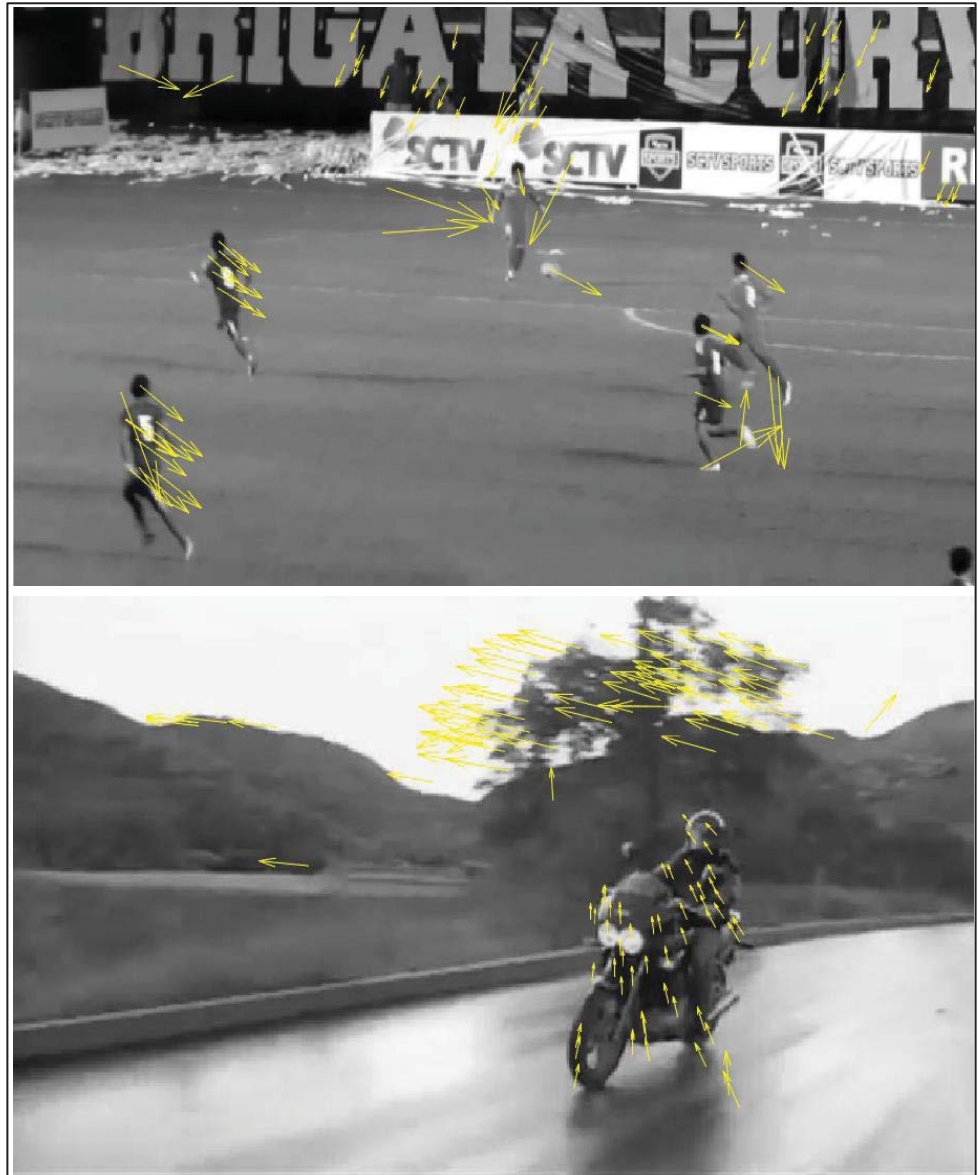
Figure 3-20: Motion vectors after elimination of outliers for Soccer frame (top) and Target frame (bottom)
