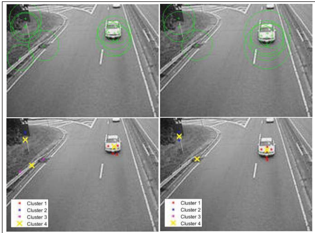
Figure 3-7: SURF feature points plotted (top row) with clustering through K-means (bottom row)
