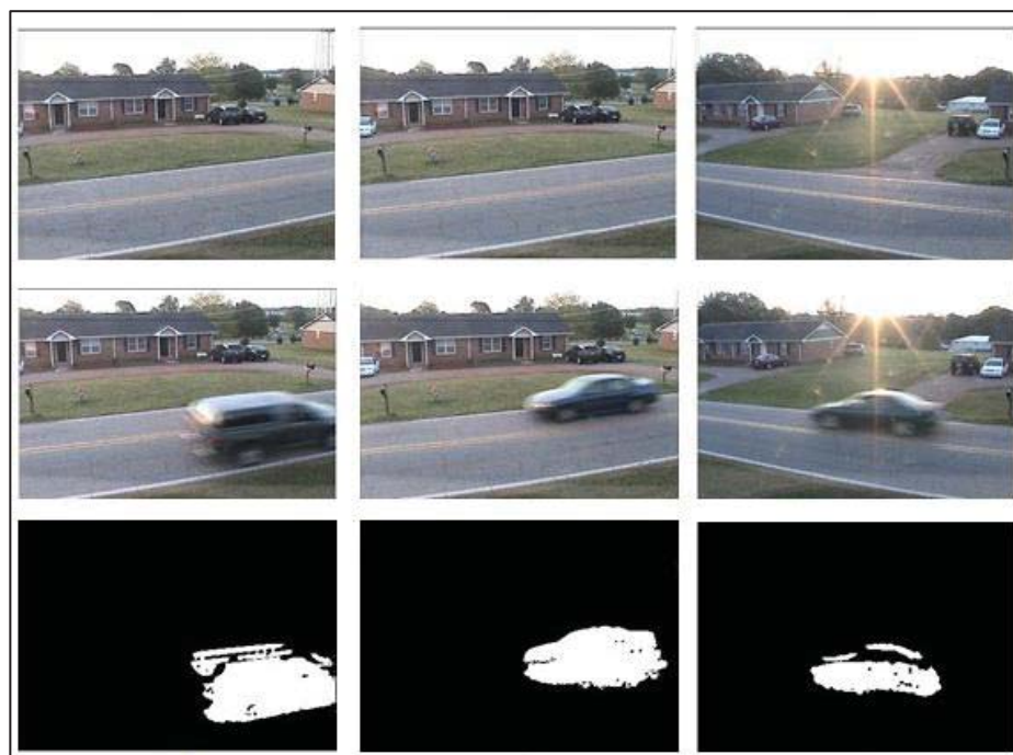
Figure 4-3: Results from [20] displays background modelling (top row), object moving in the foreground (middle row), detected object (bottom row)
