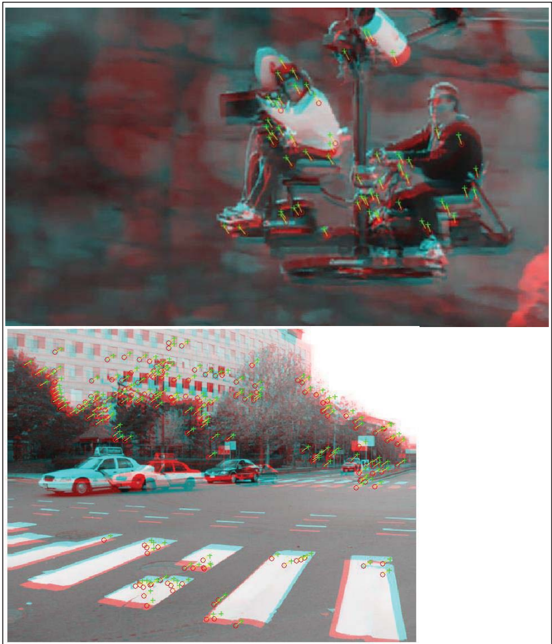
Figure 3-13: Two set of frames displaying matched feature points.
