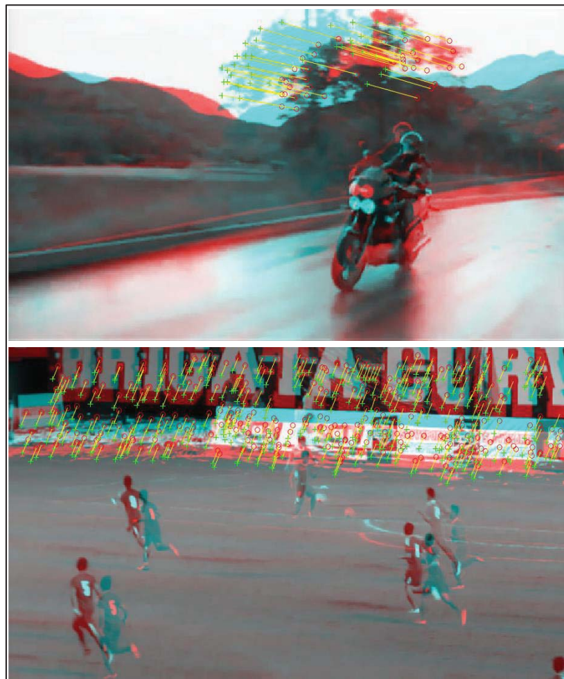
Figure 3-19: Showing pair of Target (top) and Soccer (bottom) frames depicting elimination of points using RANSAC
