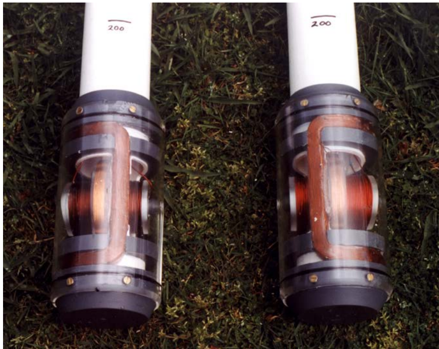
Figure 40 The coils in the probe head.
