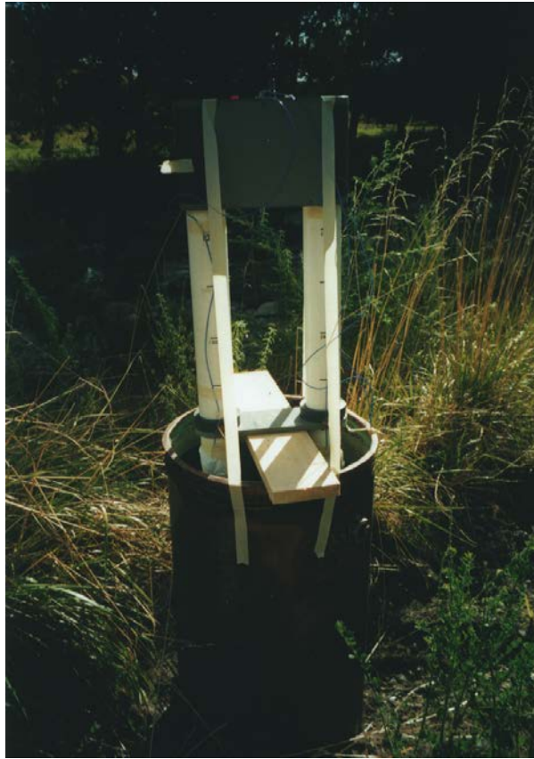
Figure 81 The large water sample experiment set up, the copper drum is filled with water.
