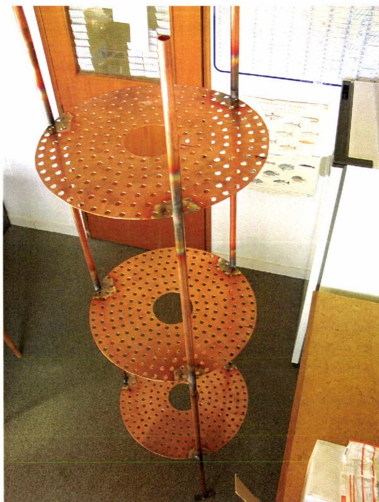
Figure 19 - The copper stand for holding the glass tubes in the water heater.
