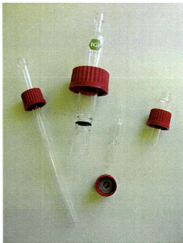
Figure 28 - The disassembled fittings of the degassing system.
