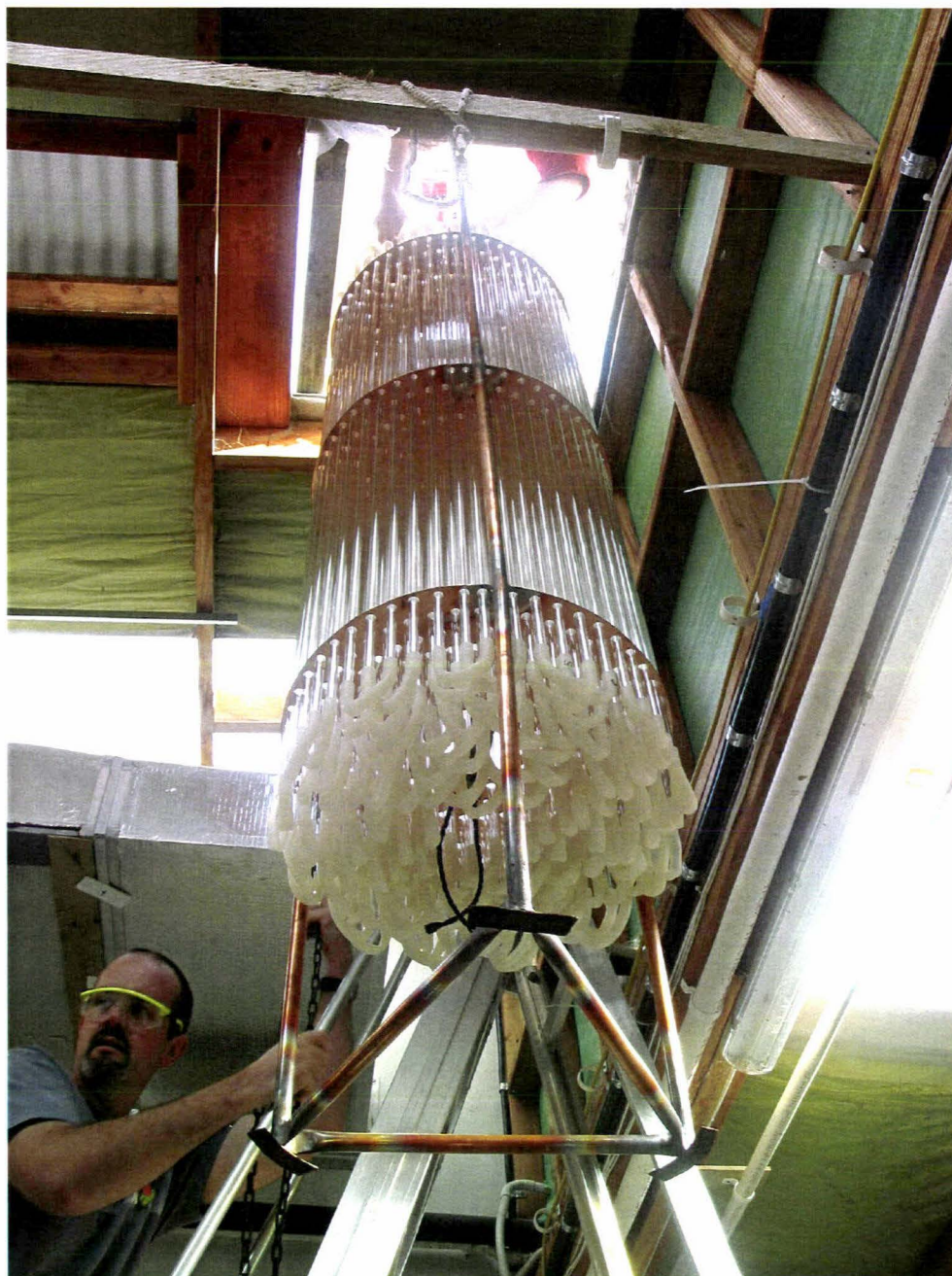
Figure 23 - The copper stand with the glass tube system lifted up so it can be lowered into the HWC. (The first trial).
